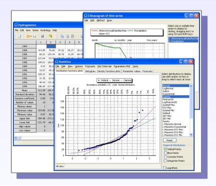
With **Hydrognomon** (see left), numerous kinds of analysis and processing of hydrological data can be performed, such as time step aggregation and regularization, interpolation, regression analysis and infilling of missing values, consistency tests, data filtering, graphical and tabular visualization of time series, statistics, and more. *Hydrognomon* is free software and the source code is available through the website of the **openmeteo.org** project.
