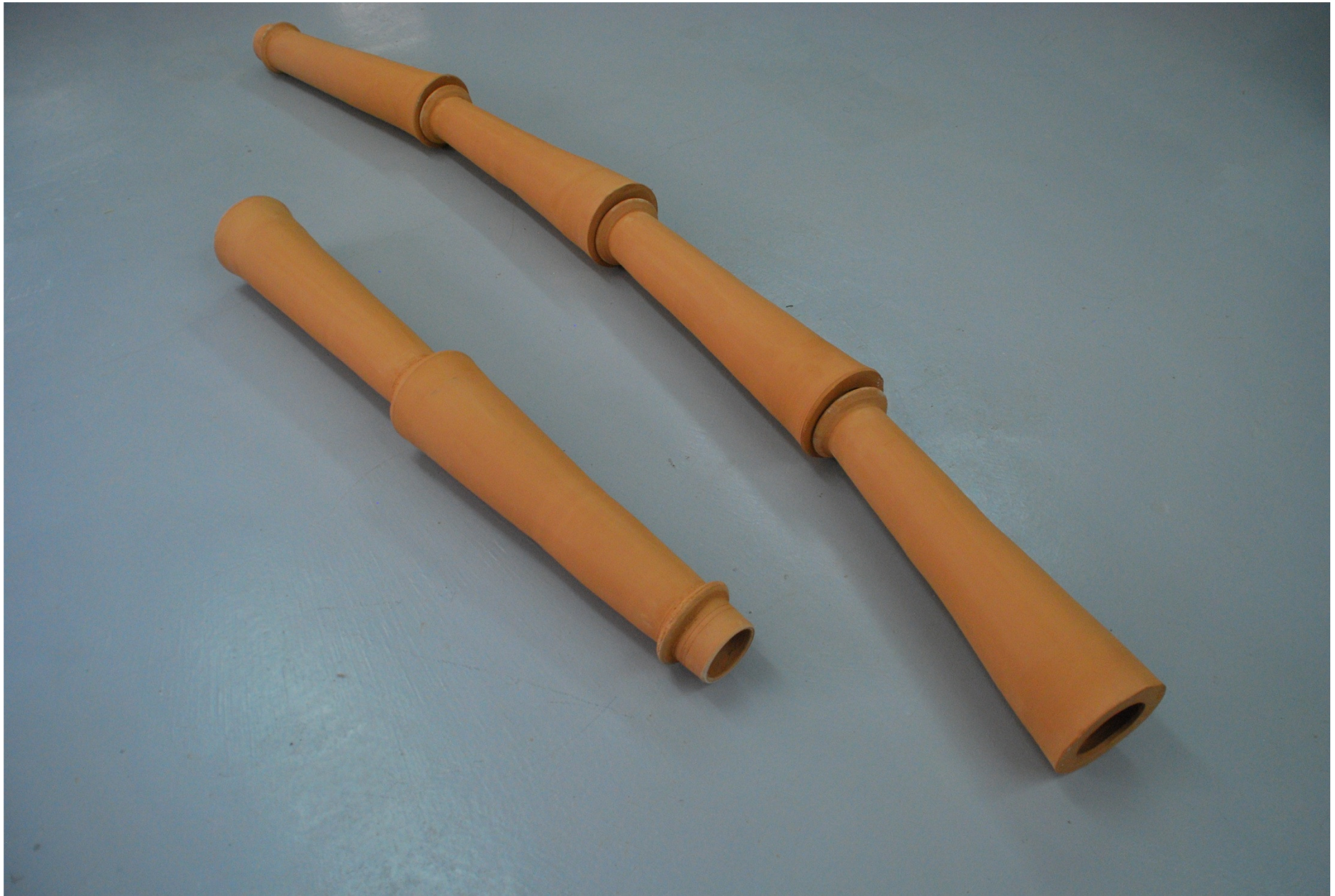
Terracotta pipes recently constructed of same material and geometry as those used at Knossos water supply system
