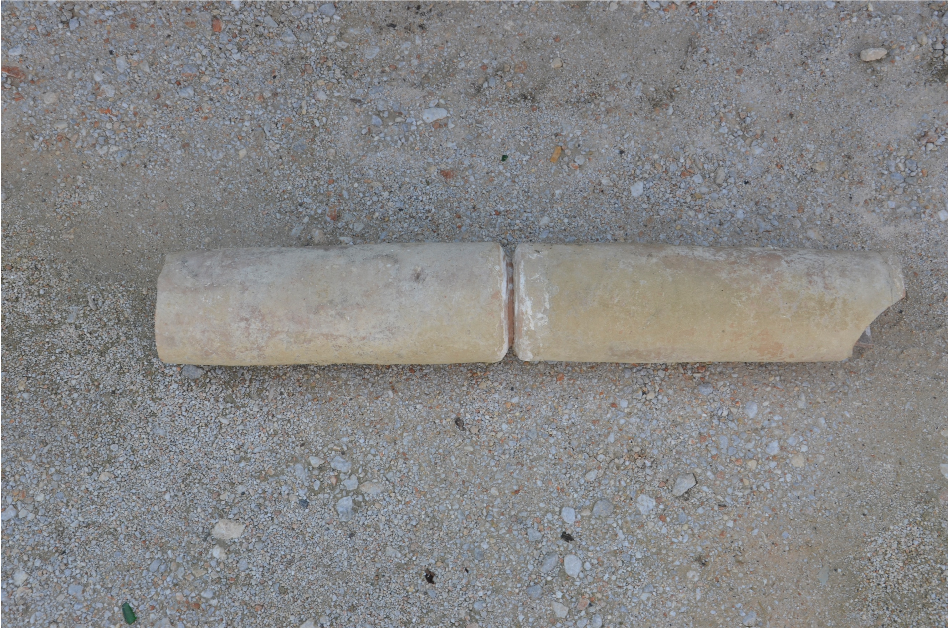
Venetian aqueduct terracotta pipe segments at Kentri in the south-eastern Crete
