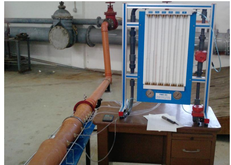
Minoan pipes at Knossos and their study at the NTUA hydraulics laboratory (Angelakis et al., 2012)
