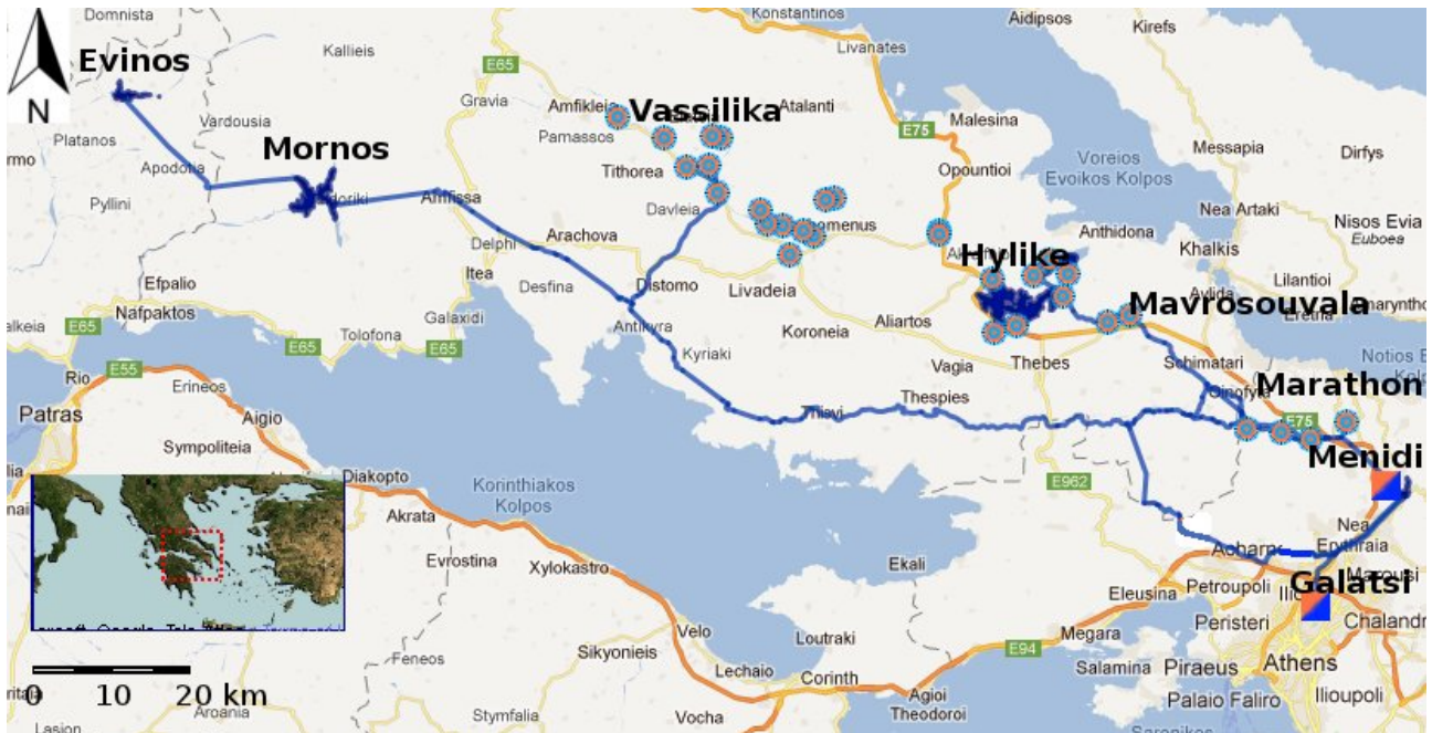
Figure 7: Athens external water supply system comprises the Evinos, Mornos, Hylike and Marathon reservoirs, the Vassilika and Mavrosouvala boreholes, and the Menidi and Galatsi treatment plants.
