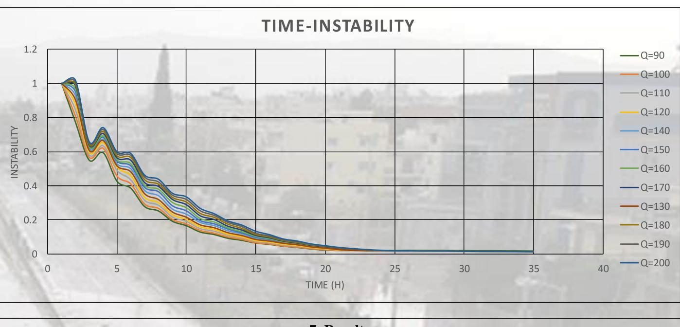
Every single discharge is assessed through comparison among the 7 pre-specified points and the water depth of simulation at each point. We used the mean square error method as a common comparative measure. Through the following Figure we were able to drew some conclusions about the steady flow estimate in between 110-120m<sup>3</sup>/s. Finally we considered that the steady state flow and the maximum observed water depth were mostly affected only by the Soures stream.
