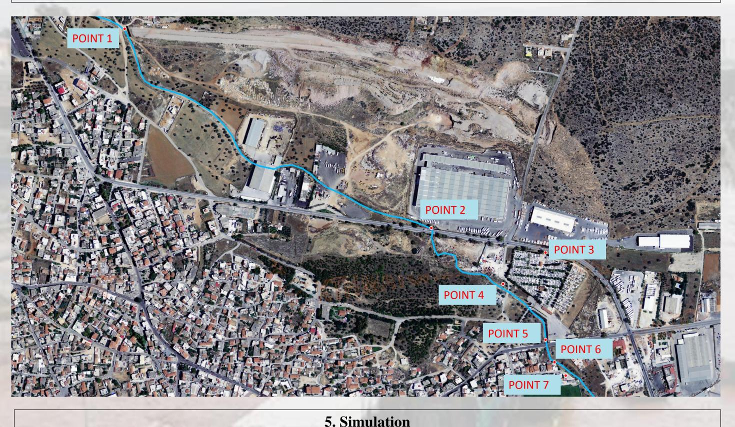
Comparing results between simulation with the quasi 2-D CFD software LISFLOOD-FP v5.9.6 and satellite reception of mapped flood extend at the area of Soures stream influence, we notice an adequate fit to the observed inundation.
