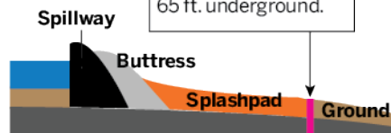
Image 34. Current repair plans for the Oroville Dam spillways. Sources: California Department of Water Resources, Bay Area News Group.
