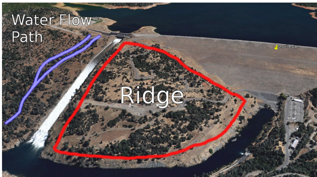
Image 35. A sketch of the ridge that protects the Oroville Dam main embankment from erosion. Adapted from Google Earth (2017).
