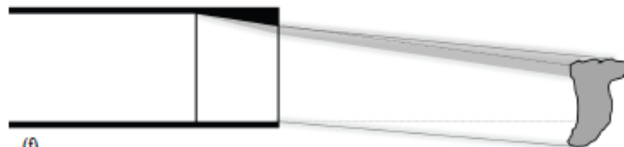
Layout 4. Vertical deflector (Juon and Hager 2000, Lucas et al. 2013, Fig. 5.6b)
