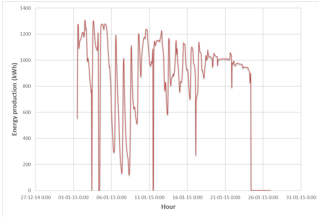
Figure 8.6: Hourly energy production through the individual operation of the Pelton turbine for one-month period.
