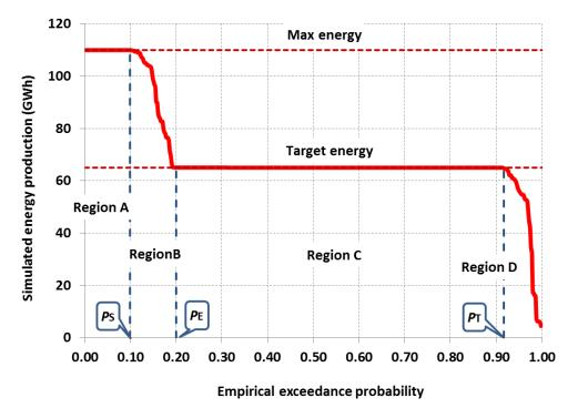
Simulated EPC at Kremasta hydroelectric reservoir, Greece, using historical inflows from 1966 to 2008 (Efstratiadis et al., 2021)
