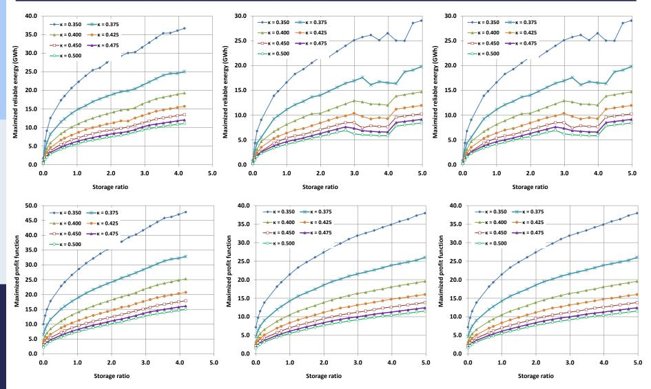
Plots of maximized energy for monthly reliability level 99% (upper panels) and maximized profit (lower panels) as function of storage ratio (storage capacity/mean annual inflow) and the shape parameter, for capacity factor CF = 80% (from left to right: Achelous, Evinos, and Boeoticos Kephisos inflow data)
