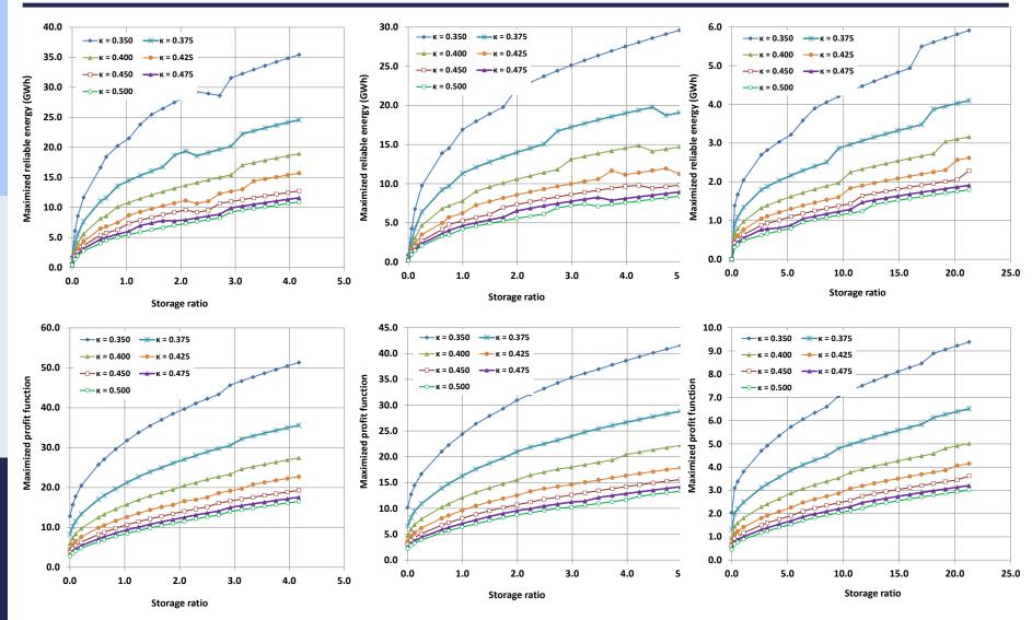
Plots of maximized energy for monthly reliability level 99% (upper panels) and maximized profit (lower panels) as function of storage ratio (storage capacity/mean annual inflow) and the shape parameter, for capacity factor CF = 20% (from left to right: Achelous, Evinos, and Boeoticos Kephisos inflow data)
