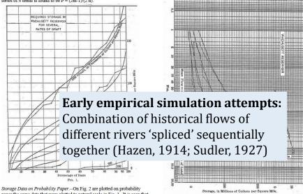
Storage Data on Probability Paper.-On Fig. 2 are plotted on probability paper the same data that were plotted to natural scale in Fig. 1. It is seen that the sharp curvature at the ends is entirely eliminated. The lines representing the several series have only a
