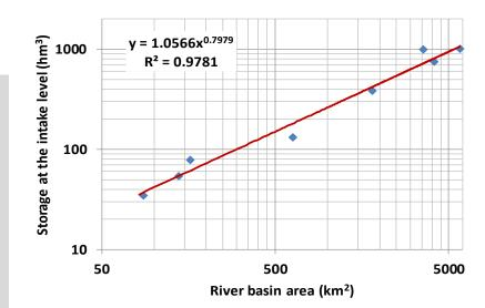
*Min. storage vs. upstream basin area, using data from eight hydroelectric reservoirs in Greece (Efstratiadis et al., 2021)*
