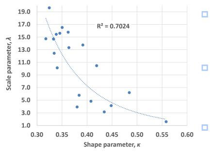
Scatter plot of shape vs. scale parameters of powertype elevation-storage function, using data from 20 large reservoirs in Greece (Efstratiadis et al., 2021)
