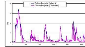
Simulation of spring discharge is good both with Darcy and Mixed equation (daily values).
