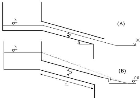
Mixed flow equation (Rozos and Koutsyiannis, 2006) resembles the function of a tunnel that discharges a reservoir. When the water level in reservoir exceeds the tunnel top, the tunnel functions like a pressurized conduit. When the water level in the reservoir is below the top, the tunnel functions like a culvert.
