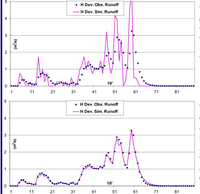
The simulated generation of runoff at the development H versus the 'observed' runoff at the output of the development H.
