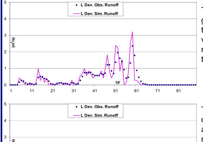
The simulated generation of runoff at the development L versus the 'observed' runoff at the output of the development L.
