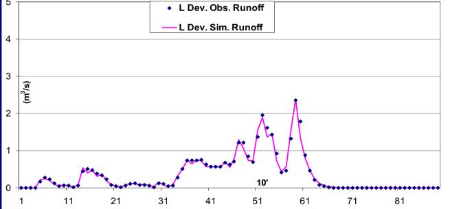
The simulated runoff at the output of the development L after the calibration of the runoff module (parameters K=3000 m<sup>3</sup> and  $\mu$  =0.50) versus the 'observed' runoff at the output of the development L.
