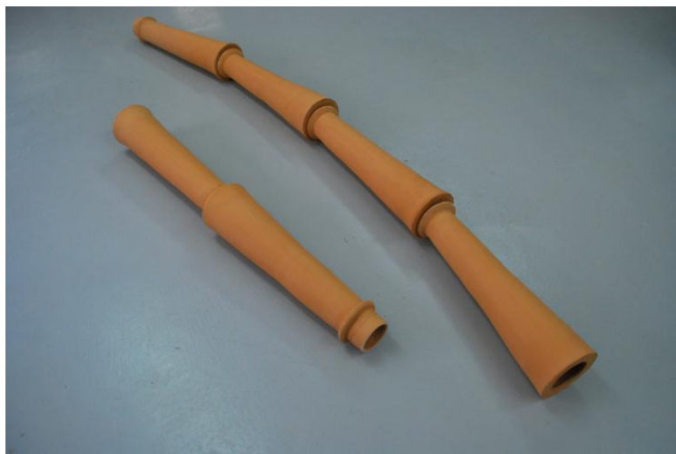
Figure 5. Knossos water supply pipes: Terracotta pipe dimensions (top) and recently constructed pipes of same material and geometry (bottom); photo by M.Nikiforakis, EFIAP with permission.
