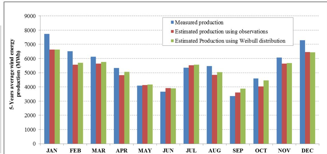
**Fig. 12:** Comparison between measured and estimated energy production (in MWh), using empirical and theoretical (Weibull) distributions applied to the selected wind turbine power curve (Pappa, 2014).
