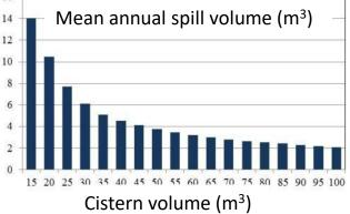
• For cistern volume 40 m<sup>3</sup>, the probability of failure (to cover demand) is less than 10%; the spill volume is about the 8% of annual potential yield.
