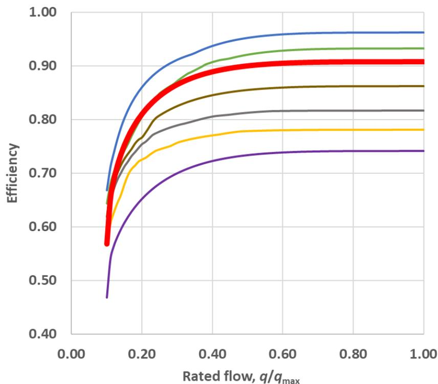
*Synthetic efficiency curves (six out of 100) around the “true” one (red line)*
