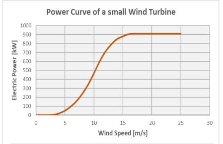
Wind energy is nonlinear transformation of wind speed, through the power curve of each specific turbine.
