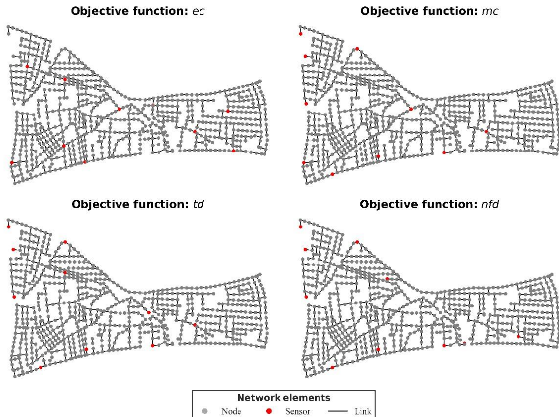
Figure 2. The four alternative sensor designs for L-Town, as generated by the respective objective functions (ObjF) from TEVA-SPOT.
