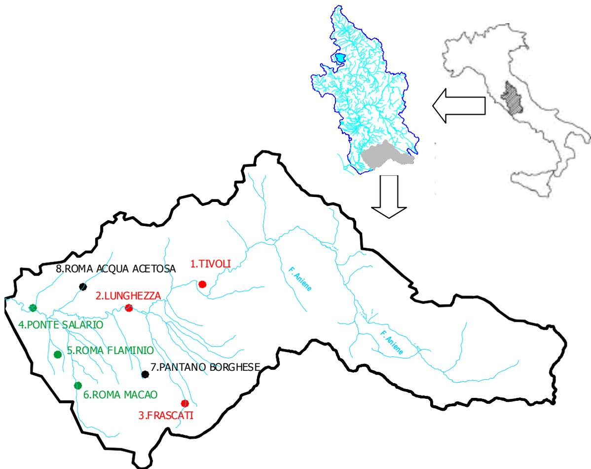
**Figure 9** Schematic of the area and the raingauges used for the case study by Futilas (2002). Gauges 1-3 are reference stations (their hourly data was used in simulation), gauges 4-6 are test stations (their hourly data was used in validation) and gauges 7-8 had only daily data.
