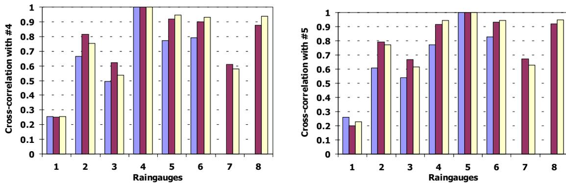
**Figure 11** Comparison of cross-correlation coefficients of hourly rainfall for the application of MuDRain at the Tiber river basin (adapted from Fytilas, 2002). In each panel, the compared values are (a) the historical value, not used in the disaggregation model; (b) the value used in the disaggregation model; (c) the synthetic value.
