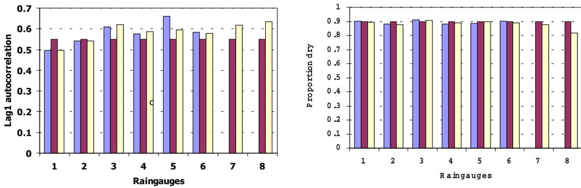
**Figure 12** Comparison of lag one autocorrelation coefficients of hourly rainfall (left) and probabilities dry (right) for the application of MuDRain at the Tiber river basin (adapted from Fytilas, 2002). In each panel, the compared values are (a) the historical value, not used in the disaggregation model; (b) the value used in the disaggregation model, which is the mean of historical values of gauges 1-3; (c) the synthetic value.
