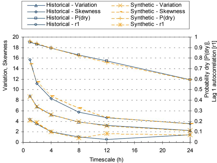
**Figure 6** Comparison of coefficient of variation and skewness, probability of dry intervals and lag one autocorrelation coefficient of historical and synthetic data at timescales (aggregation levels) 1 to 24 hours for the case study of Walnut Gulch Gauge 13, month of July (Koutsoyiannis and Onof, 2001).
