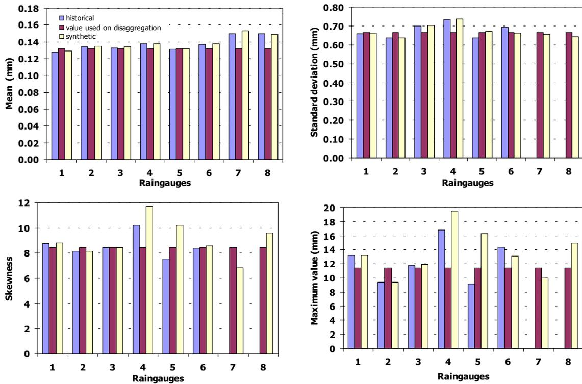
**Figure 10** Comparison of marginal statistics of hourly rainfall for the application of MuDRain at the Tiber river basin (adapted from Fytilas, 2002). In each panel, the compared values are (a) the historical value, not used in the disaggregation model; (b) the value used in the disaggregation model, which is the mean of historical values of gauges 1-3; (c) the synthetic value.
