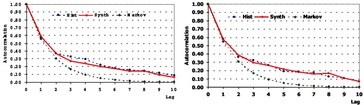
**Figure 13** Comparison of autocorrelation functions of hourly rainfall for the application of MuDRain at the Tiber river basin (adapted from Fytilas, 2002), as determined from historical or simulated series, or theoretically implied from the AR(1) (Markov) model, for gauges 4 (left) and 6 (right).
