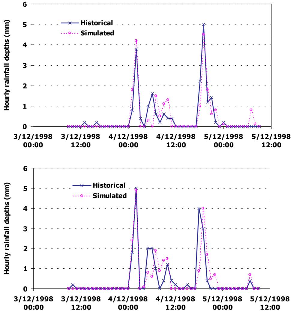
**Figure 15** Comparison of historical and simulated hyetographs from the application of MuDRain at the Tiber river basin at a day with high rainfall for gauges 4 (upper panel) and 6 (lower panel) (adapted from Fytilas, 2002).
