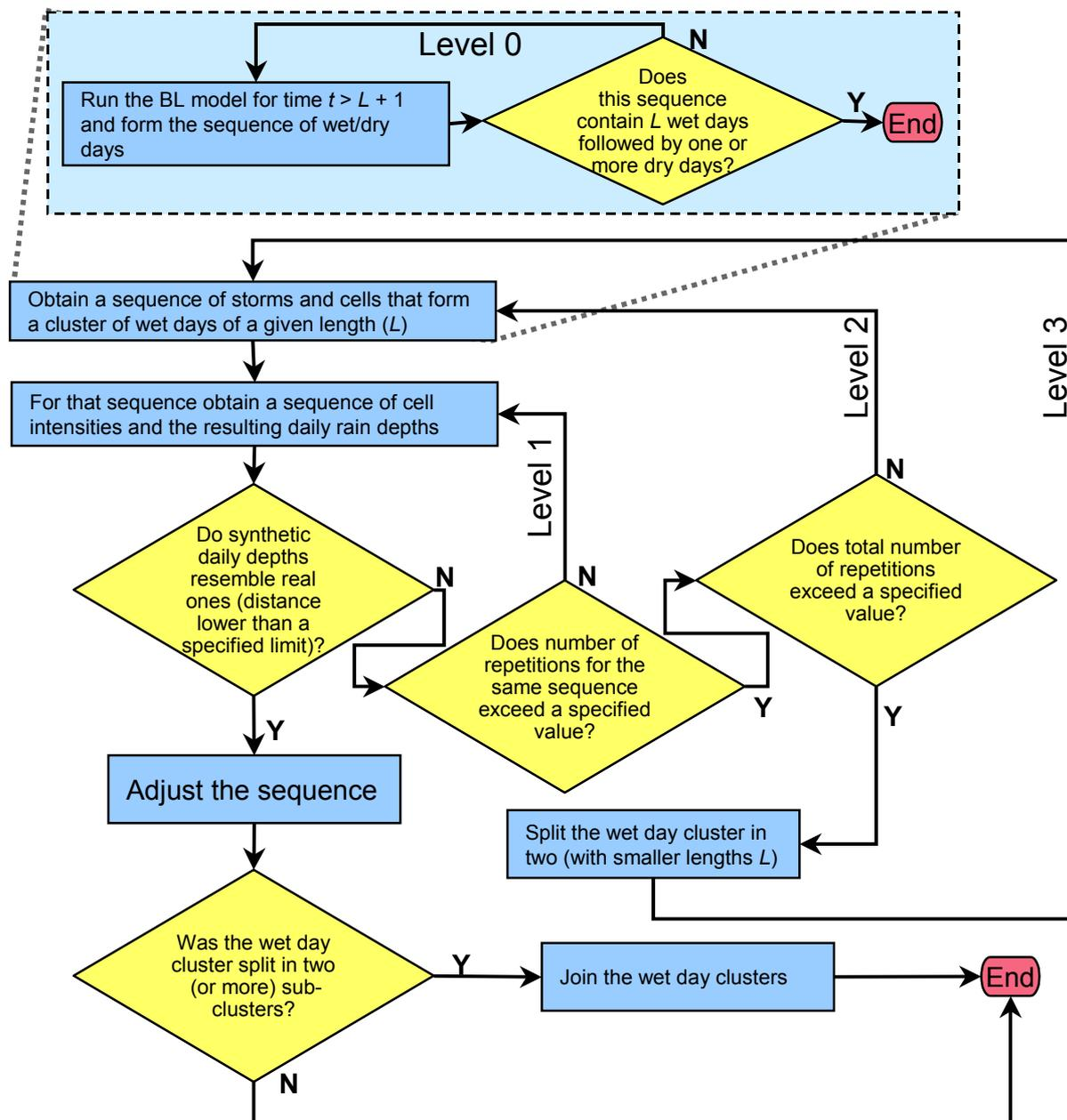
Figure 1 Flow diagram of the repetition scheme used in Hyetos (Koutsoyiannis and Onof, 2001).
