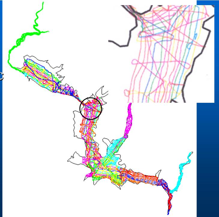
Determination of reservoir segments with sediment deposits
