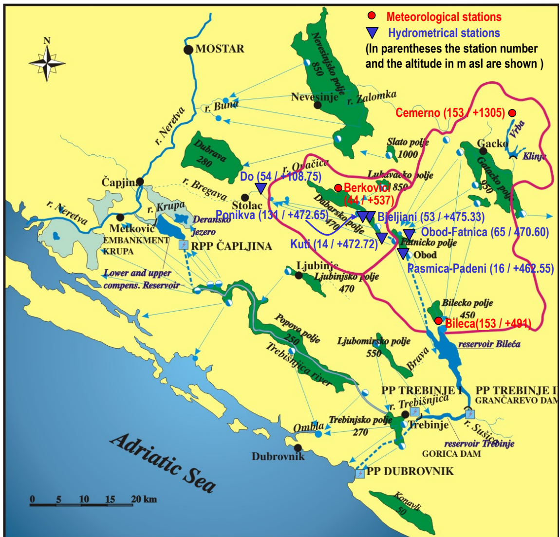
Figure 76. General layout of the hydrosystem of Trebišnjica and Bregava river catchments with the karstic fields, the natural hypothetical connections, the artificial tunnels and the locations of meteorological and hydrometrical stations.
