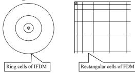
In the case of isotropic aquifer, IFDM gave more accurate results (see Table) and was much faster (10 instead of 10x10 cells) than FDM.
