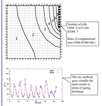
In terms of time series of hydraulic heads the determination coefficient expressing the difference of the two models varies from 0.85 to 0.95\* (FDM cells are grouped according to the corresponding IFDM discretisation in 7 groups, the heads of cells in each group are aggregated resulting in 7 time series).
