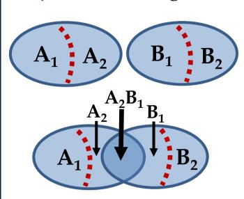
Independent energy systems A+B Efficiency:  $(A_1+B_1)/(A+B)$ Losses:  $(A_2 + B_2)/(A + B)$ , with  $[A_1 | B_2] = [B_1 | A_2] = \emptyset$ **Integrated energy systems A+B** Efficiency:  $(A_1+B_1)/(A+B)$ Losses:  $(A_2+B_2-A_2B_1)/(A+B)$ Efficiency increase due to system integration  $(A_2+B_2)/(A+B) > (A_2+B_2-A_2B_1)/(A+B)$
