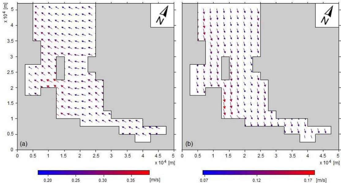
**Figure 5.** Izmir Bay surface currents for (a) E wind – 4 bf, (b) NW wind – 2 bf.
