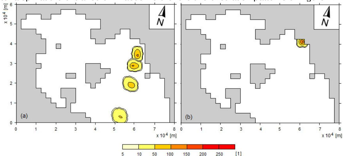
**Figure 3.** Saronikos Gulf oil slick trajectories for (a) N wind – 4 bf, (b) S wind – 3 bf.
