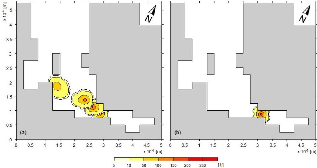
**Figure 7.** Izmir Bay oil slick trajectories for (a) E wind – 4 bf, (b) NW wind – 2 bf.
