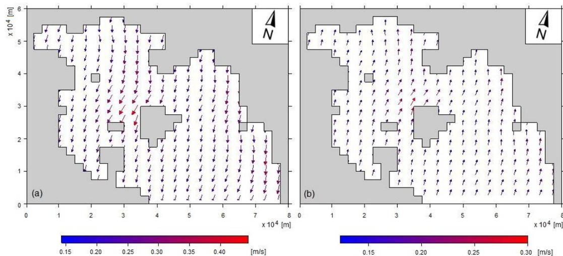
**Figure 1.** Saronicos Gulf surface currents for (a) N wind – 4 bf, (b) S wind – 3 bf.
