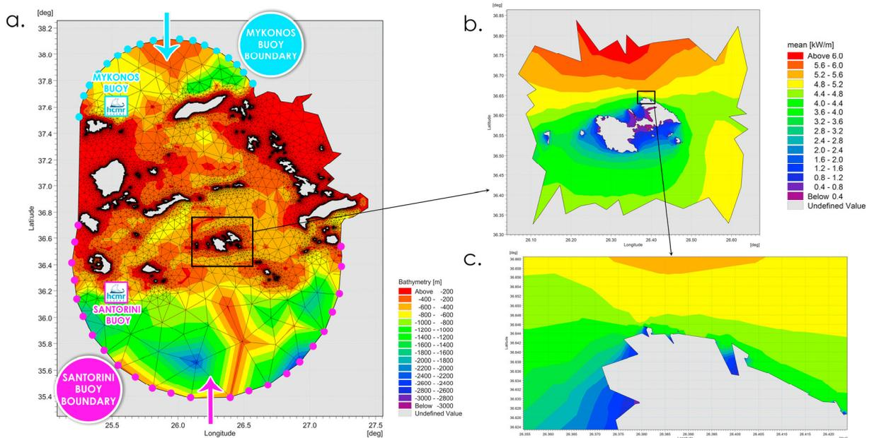
Figure 1. (a) Initial bathymetry and mesh of the MIKE 21 SW model. Location of buoys and open boundaries; (b) Mean Wave Power [kW/m] results around Astypalaia from MIKE 21 SW model; (c) Mean Wave Power [kW/m] results around the WEC installation point.
