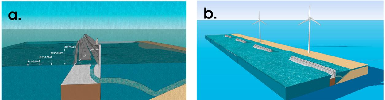
Figure 4. (a) Schematic representation of the Overtopping Wave Energy converter simulated in this study; (b) Schematic representation of the Hybrid Renewable Energy System designed for the case study, containing two wind turbines and four overtopping wave energy converters.
