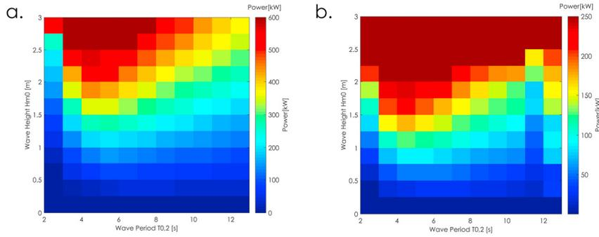
Figure 3. Power matrices of (a) the prototype 600 kW Wave Star WEC; (b) the downscaled 250 kW Wave Star WEC
