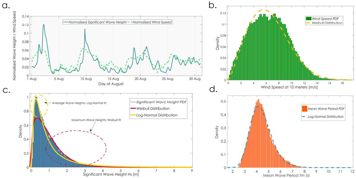
Figure 2. (a) A monthly (August) window of normalised wind and wave resources. Distribution fitting for (b) Wind Speed at 10 meters ( $U_{10}$ ); (c) Significant Wave Height ( $H_s$ ); (d) Mean Wave Period ( $T_m$ )
