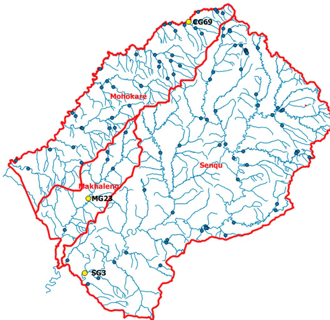
**Figure 1.** Catchment boundaries (red lines), hydrographic network and flow monitoring stations (blue points) across Lesotho (the three pilot stations are highlighted in yellow).
