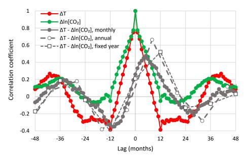
**Figure 14.** Auto- and cross-correlograms of the differenced time series of UAH temperature and Mauna Loa CO<sub>2</sub> concentration.
