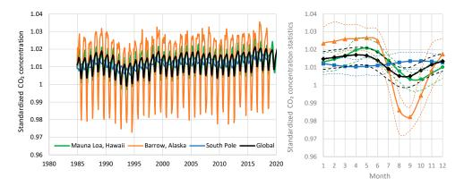
**Figure 7.** Plots of atmospheric  $CO_2$  concentration after standardization: (**left**) each monthly value is standardized by dividing with the geometric average of the 5-year period before it. (**right**) Monthly statistics of the values of the left panel; for each month the average is shown in continuous line and the minimum and maximum in thin dashed lines of the same colour as the average.
