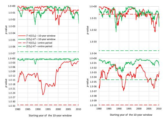
**Figure 10.** Plots of *p*-values of the Granger test for 10-year-long moving windows for the monthly time series of UAH temperature and logarithm of CO<sub>2</sub> concentration at Mauna Loa for number of lags (**left**)  $\eta = 1$  and (**right**)  $\eta = 2$ . The time series used are: (**upper**) the original, and (**lower**) the obtained after "removing" the periodicity by averaging over the previous 12 months.
