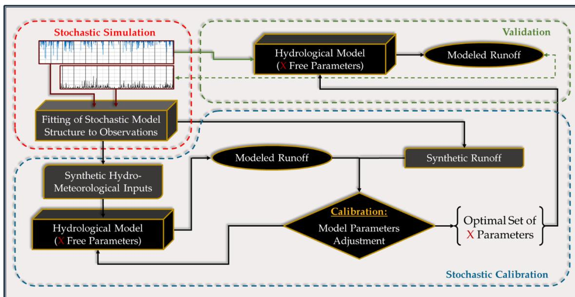
**Figure 3.2** | Schematic representation of the conceptual structure of stochastic calibration
