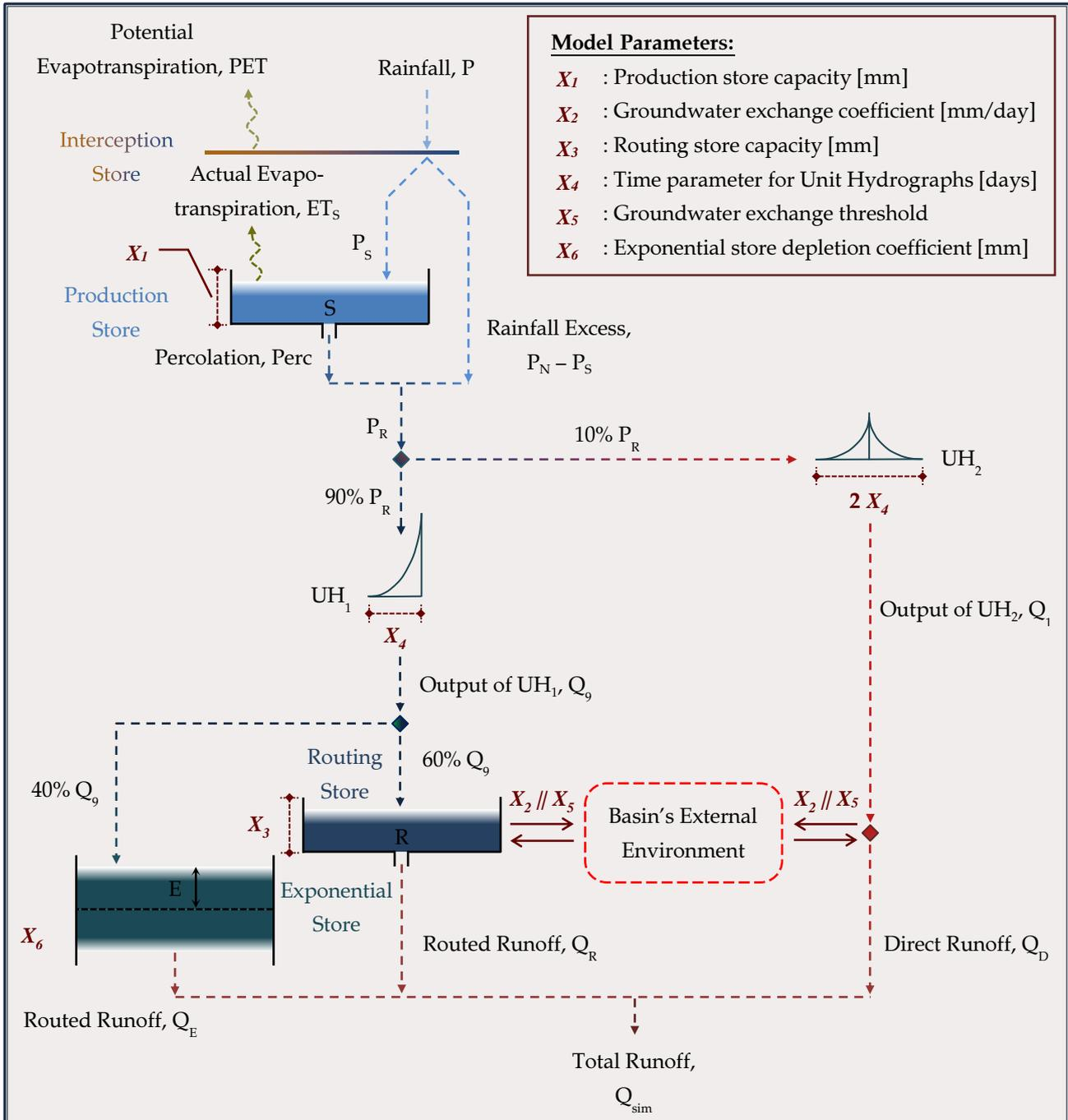
Figure 4.5 | Schematic representation of the conceptual structure of the GR6J model
