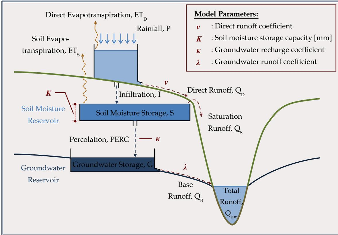
**Figure 4.1** | Schematic representation of the conceptual structure of the Zygos4P
