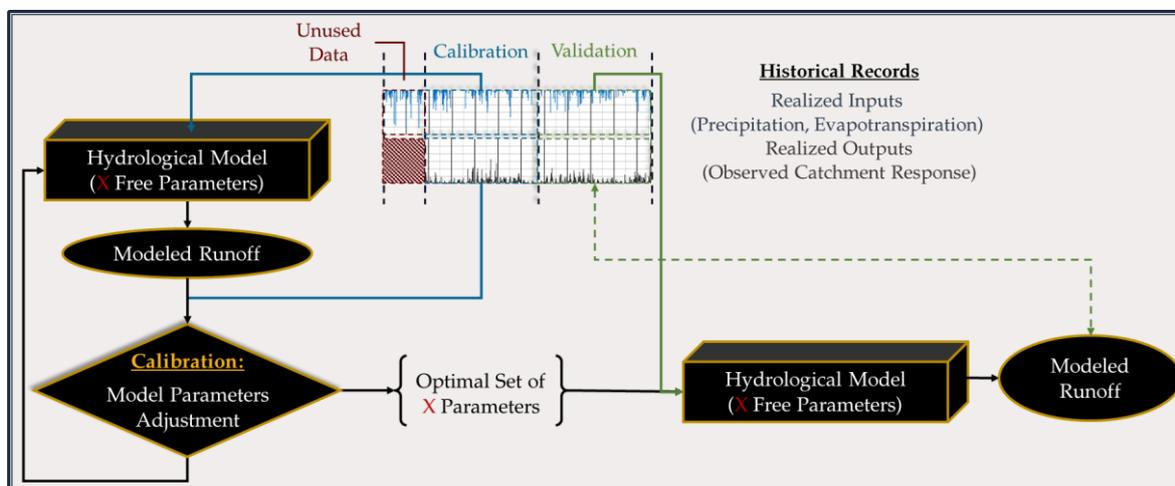
**Figure 3.1** | Schematic representation of the classical split-sample scheme
