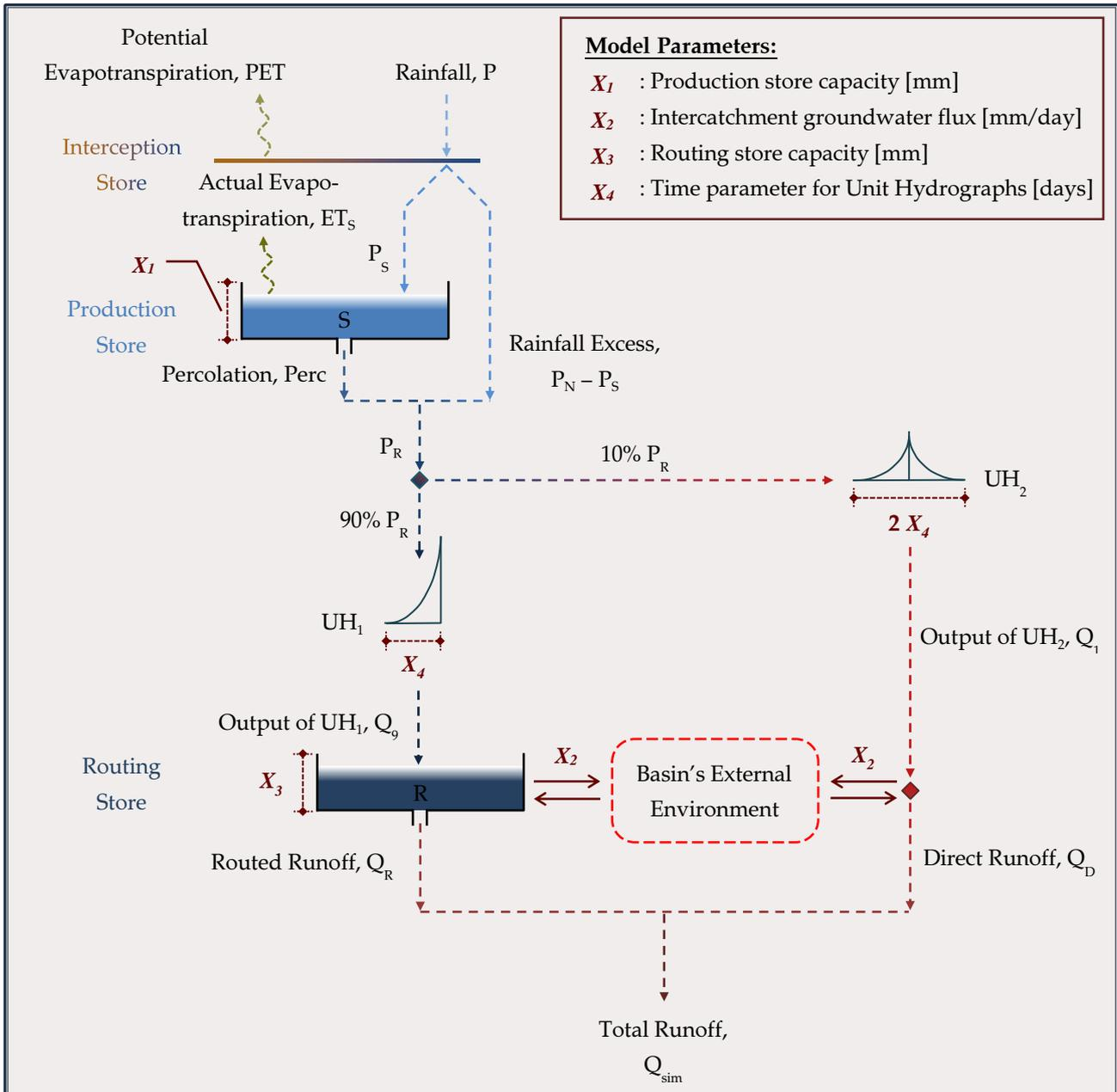
**Figure 4.4** | Schematic representation of the conceptual structure of the GR4J model
