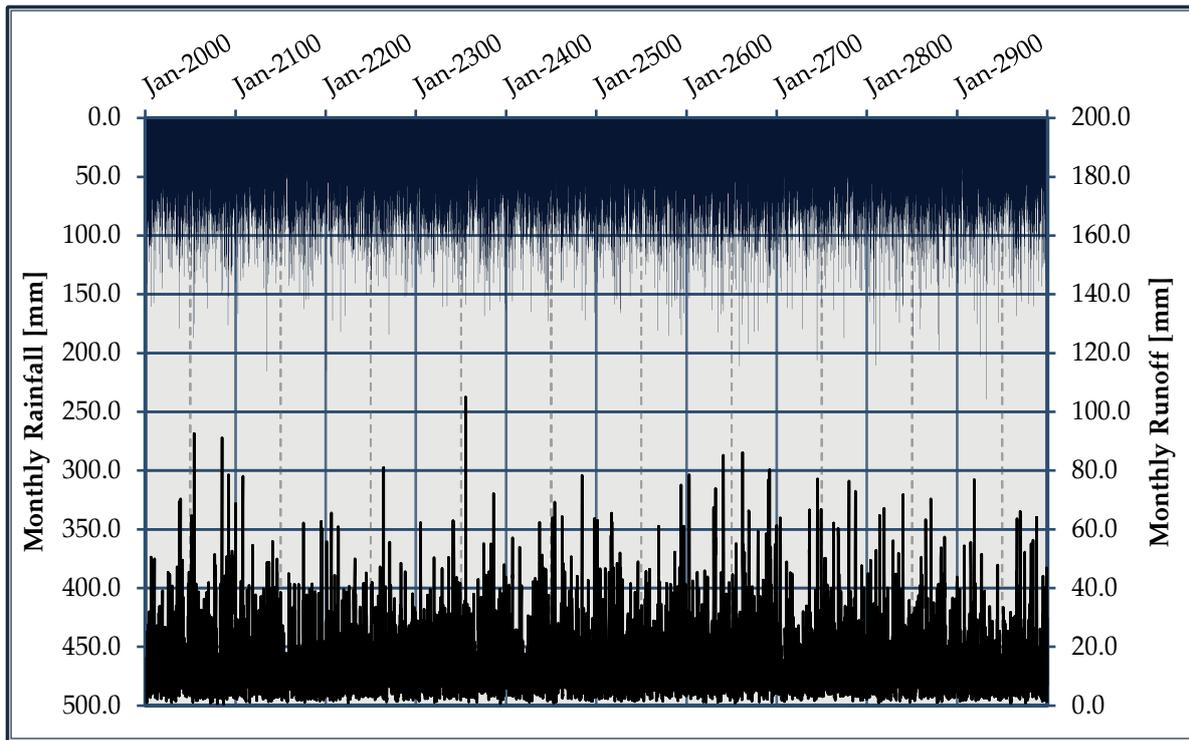
Figure 5.4 | Synthetically generated rainfall and runoff time series (randomly selected window of 1000 years)
