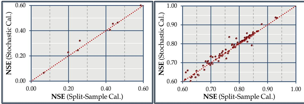
**Figure 6.2** | Scatter plots of poor/low (left) or good/high (right) model performance (NSE) by employing the Split-Sample approach and the Stochastic Calibration (GR2M model)
