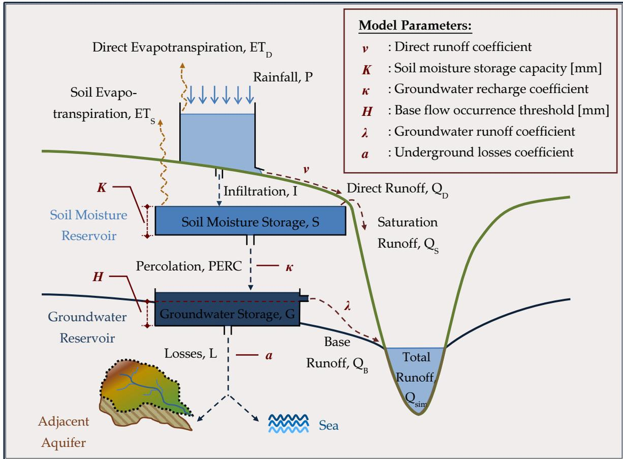
**Figure 4.2** | Schematic representation of the conceptual structure of the Zygos6P
