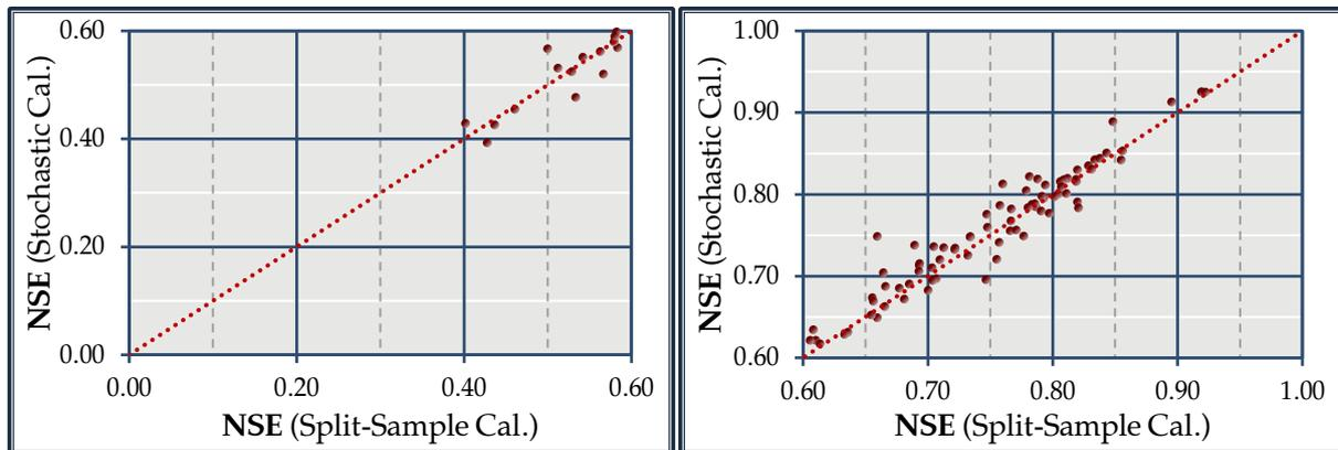
**Figure 6.6** | Scatter plots of poor/low (left) or good/high (right) model performance (NSE) by employing the Split-Sample approach and the Stochastic Calibration (Zygos6P model)
