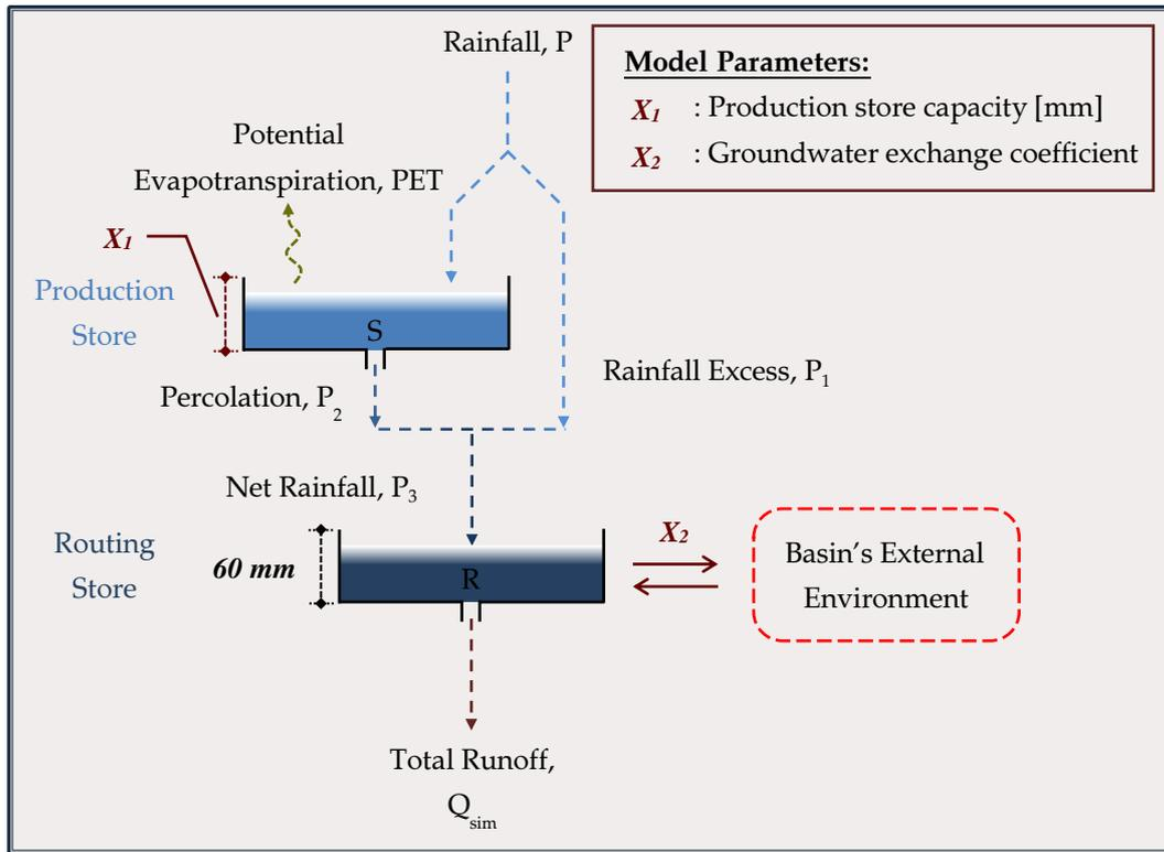
**Figure 4.3** | Schematic representation of the conceptual structure of the GR2M model
