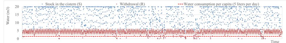
Considering R=6 m³ the average consumption is 4.2m³ per month and the system failure is about 7.2%
