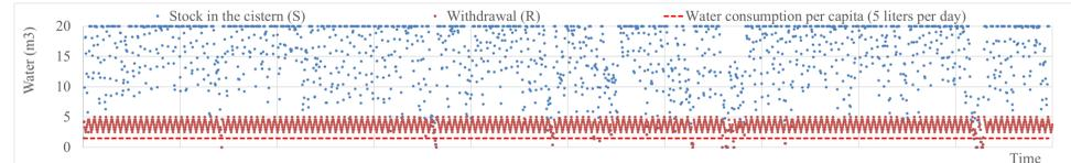
Considering R=5 m³ the average consumption is 3.7m³ per month and the system failure is about 3.8%
