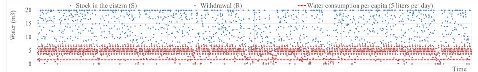
Considering R=7 m³ the average consumption is 4.6m³ per month and the system failure is about 15%
