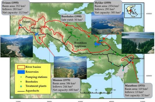
Hylike is a natural lake, lying in a karstic background, and may lose half of its storage capacity in one year due to leakages
