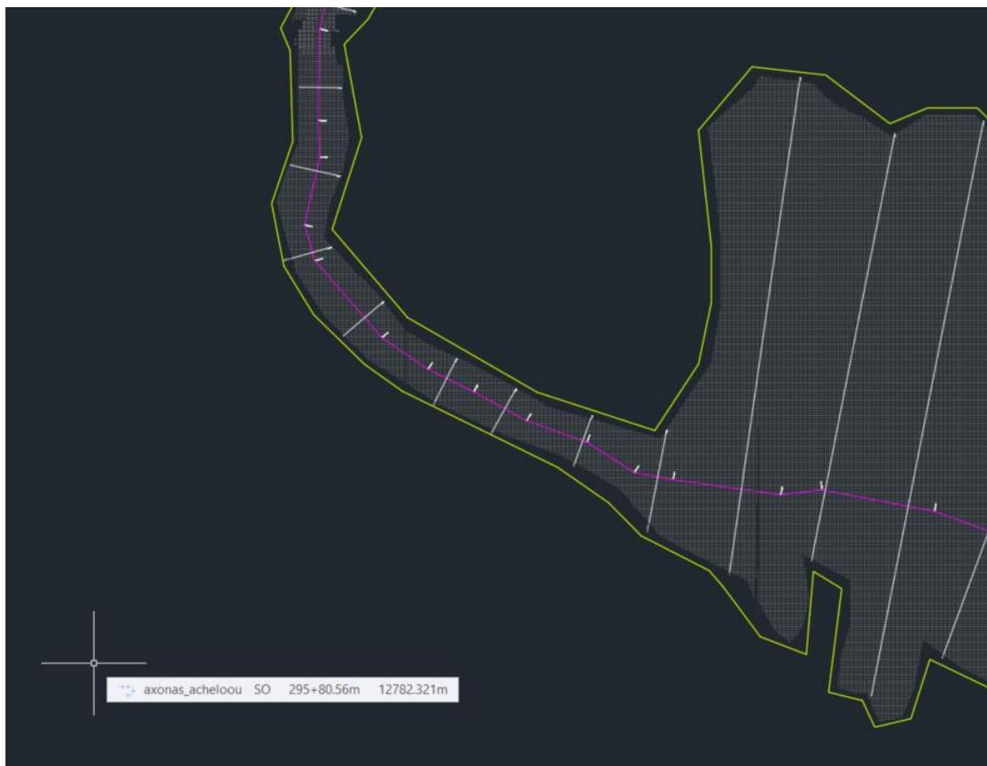
**Figure 5.2-5:** “Alignment” and “Sample Lines” (Civil 3D 2019)
