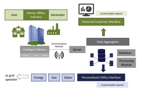
Fig. 1. Digital multi-utility system architecture overview.
