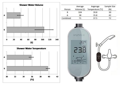
Fig. 5. Summary results for volume and temperature for Persons A and B (Amphiro meter).
