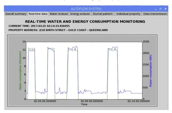
Fig. 2. Concurrent water-electricity demand signal (5s; L/min and Wh) (Autoflow screen shot).
