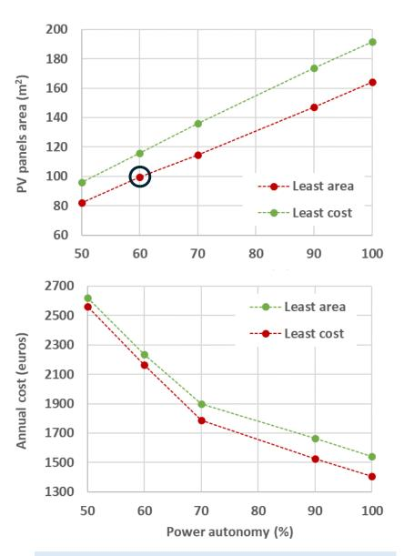
Graphs of the cost and PV panel area with respect to SM unit power autonomy for the two optimization scenarios (least area, least cost).
