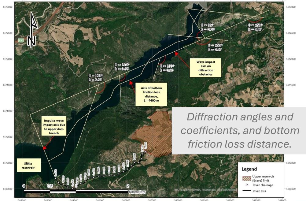
Diffraction angles and coefficients, and bottom friction loss distance.
