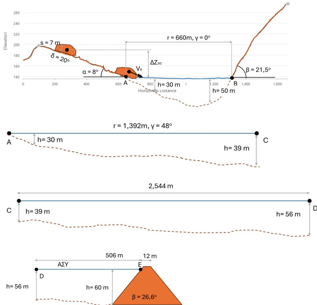
Layout of cross-sections AB, AC, CD, and DE (from top to bottom).
