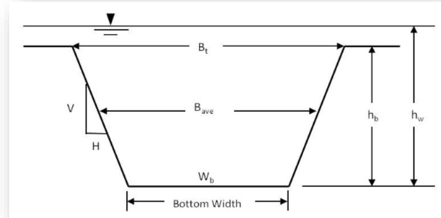
Typical breach parameters (model assumptions)
