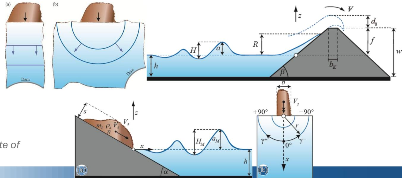
Geometry of Sfikia reservoir and characteristic points illustrating the route of the wave produced by the water volume arriving at point A
