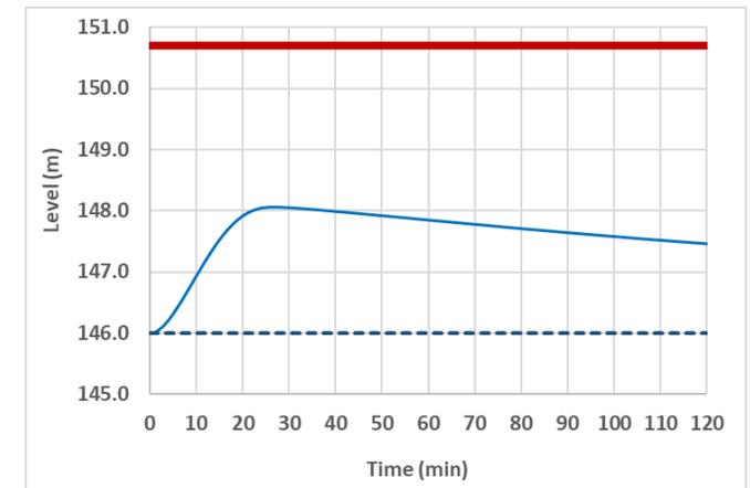
Time series of inflows vs. routed outflows (left) and reservoir level (right) for scenarios 1 (upper panel) and 4 (lower panel). The red line indicates the dam crest.
