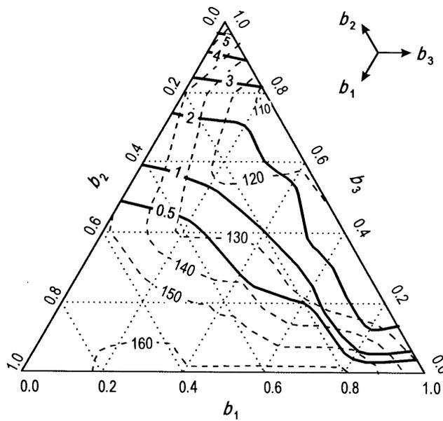
**Figure 4.** Contours of equal probability of failure  $\alpha'$  (%) of the Athens water supply system (solid lines) and of equal mean annual abstraction from Lake Iliki  $E[R_3]$  in cubic hectometers (dashed lines) for the first (coarsest) grid of the optimization process in problem 2. The annual target release is  $600 \text{ hm}^3$ . Parameters  $a_i$  are zero for all reservoirs.
