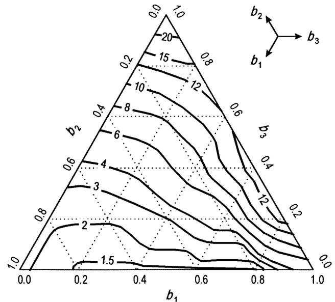
**Figure 3.** Contours of equal probability of failure  $\alpha'$  (%) of the Athens water supply system for the first (coarsest) grid of step 1 of the optimization process of problem 1. The annual target release is  $700 \text{ hm}^3$ . Parameters  $a_i$  are zero for all reservoirs.
