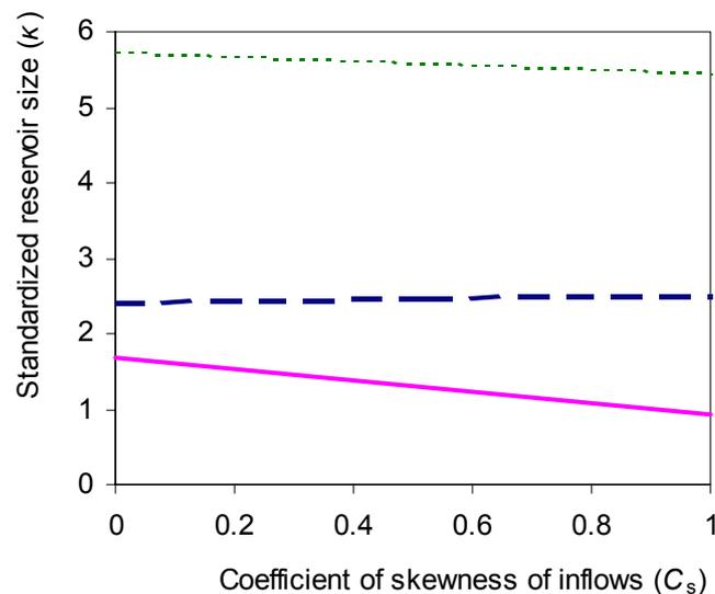
**Figure 3** Effect of the skewness of inflows to the standardized reservoir size ( $\kappa$ ) required to achieve a drift  $\varepsilon = 0.8$  with a reliability level  $\alpha = 98\%$  (continuous line), a drift  $\varepsilon = 0.2$  with a reliability level  $\alpha = 90\%$  (dashed line), and a drift  $\varepsilon = 0.2$  with a reliability level  $\alpha = 98\%$  (dotted line). Results are obtained by simulation using independent two-parameter gamma distributed inflows.
