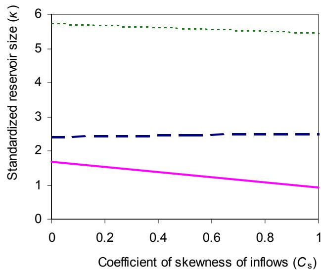
**Figure 3** Effect of the skewness of inflows to the standardized reservoir size ( $\kappa$ ) required to achieve a drift  $\varepsilon = 0.8$  with a reliability level  $\alpha = 98\%$  (continuous line), a drift  $\varepsilon = 0.2$  with a reliability level  $\alpha = 90\%$  (dashed line), and a drift  $\varepsilon = 0.2$  with a reliability level  $\alpha = 98\%$  (dotted line). Results are obtained by simulation using independent two-parameter gamma distributed inflows.
