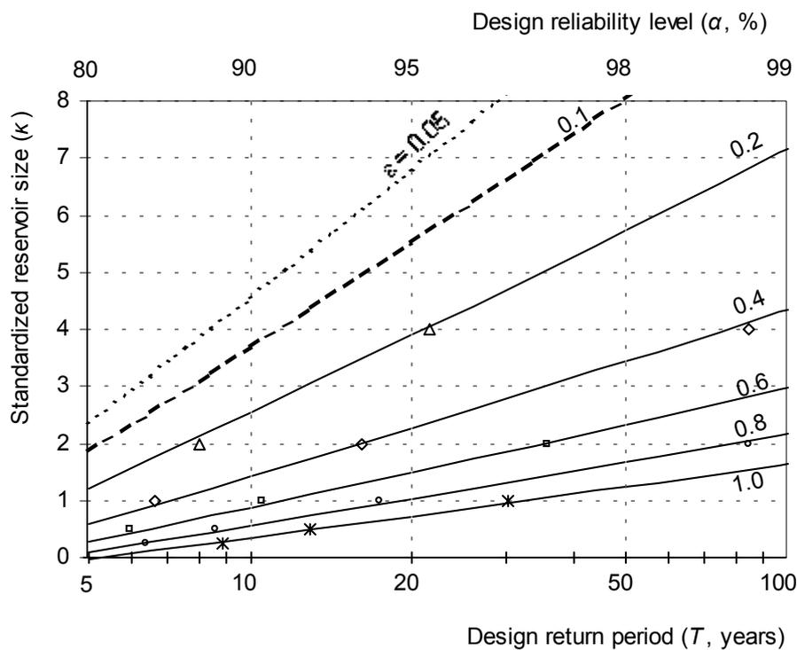
**Figure 1** A simple representation of reservoir size-yield-reliability: Standardized reservoir size ( $\kappa = K / \sigma$ ) required to achieve a certain drift ( $\varepsilon = (\mu - \delta)/\sigma$ ) with a certain reliability level, for independent inputs normally distributed. Lines are constructed from equation (20) whereas plotted points are theoretical results by Pegram (1980) for  $\varepsilon = 0.2$  (triangles), 0.4 (diamonds), 0.6 (squares), 0.8 (circles) and 1.0 (stars).
