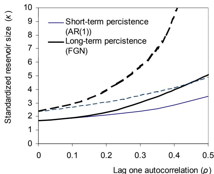
**Figure 2** Effect of short-term and long-term hydrologic persistence of inflows to the standardized reservoir size ( $\kappa$ ) required to achieve a drift  $\varepsilon = 0.8$  with a reliability level  $\alpha = 98\%$  (continuous lines) and a drift  $\varepsilon = 0.2$  with a reliability level  $\alpha = 90\%$  (dashed lines). Results are obtained by simulation.
