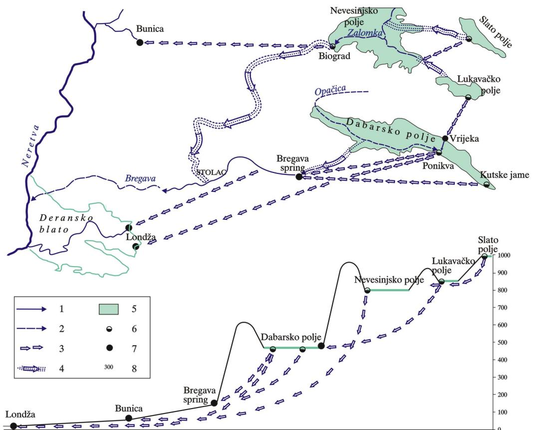
**Figure 21.** Break-up of surface river network of the Bregava River basin as a result of the evolution of processes (Milanović, 1981)
