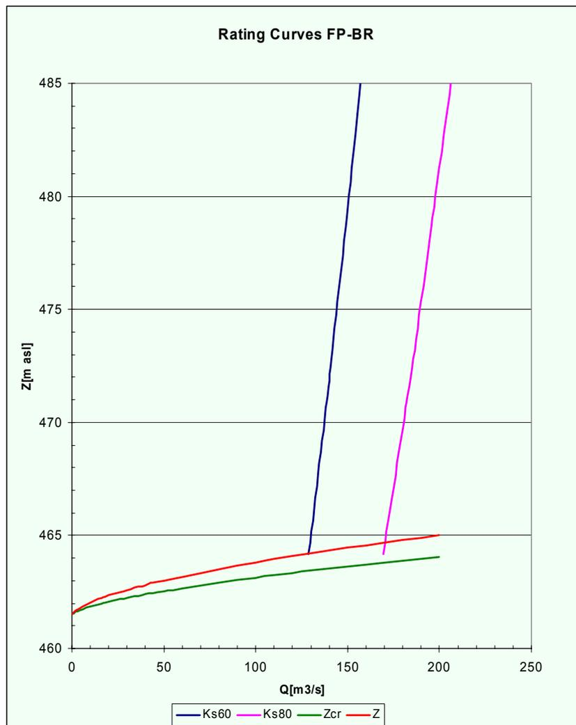
**Figure 9.** Capacity of the tunnel between Fatničko polje and Bileća reservoir
