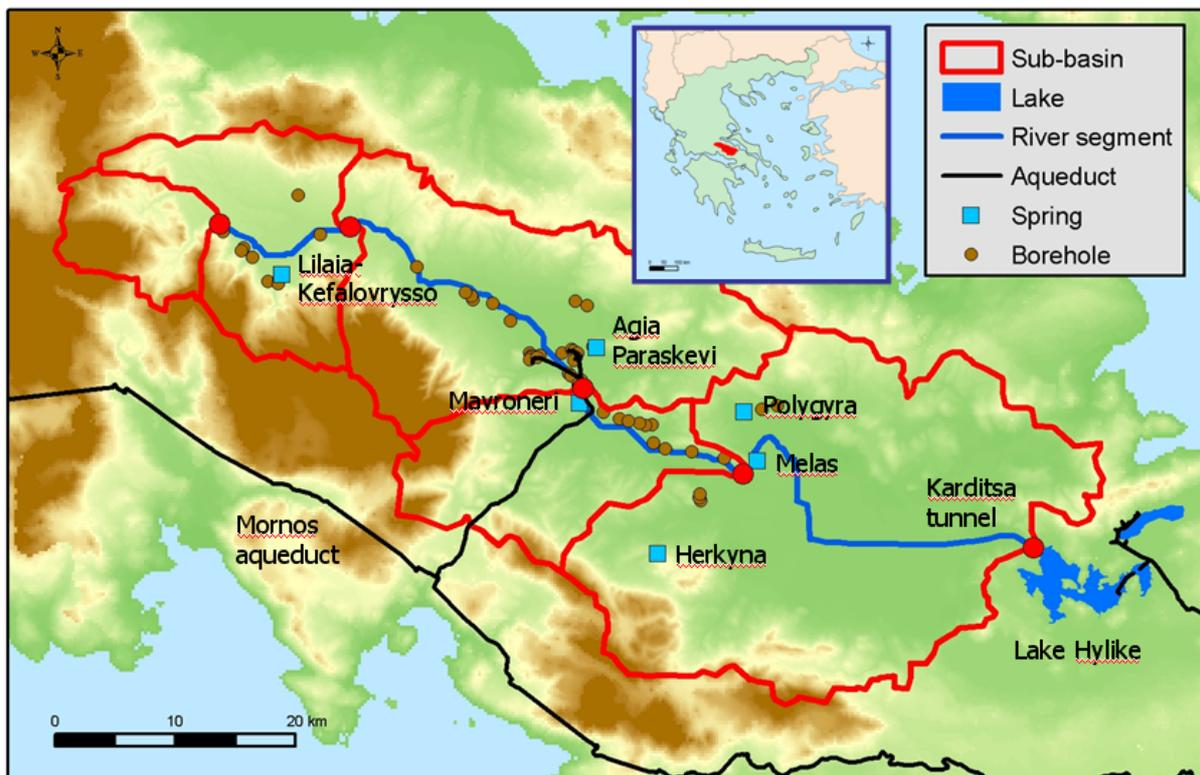
Figure 3: The Boeotikos Kephisos river basin and the main hydrosystem components.
