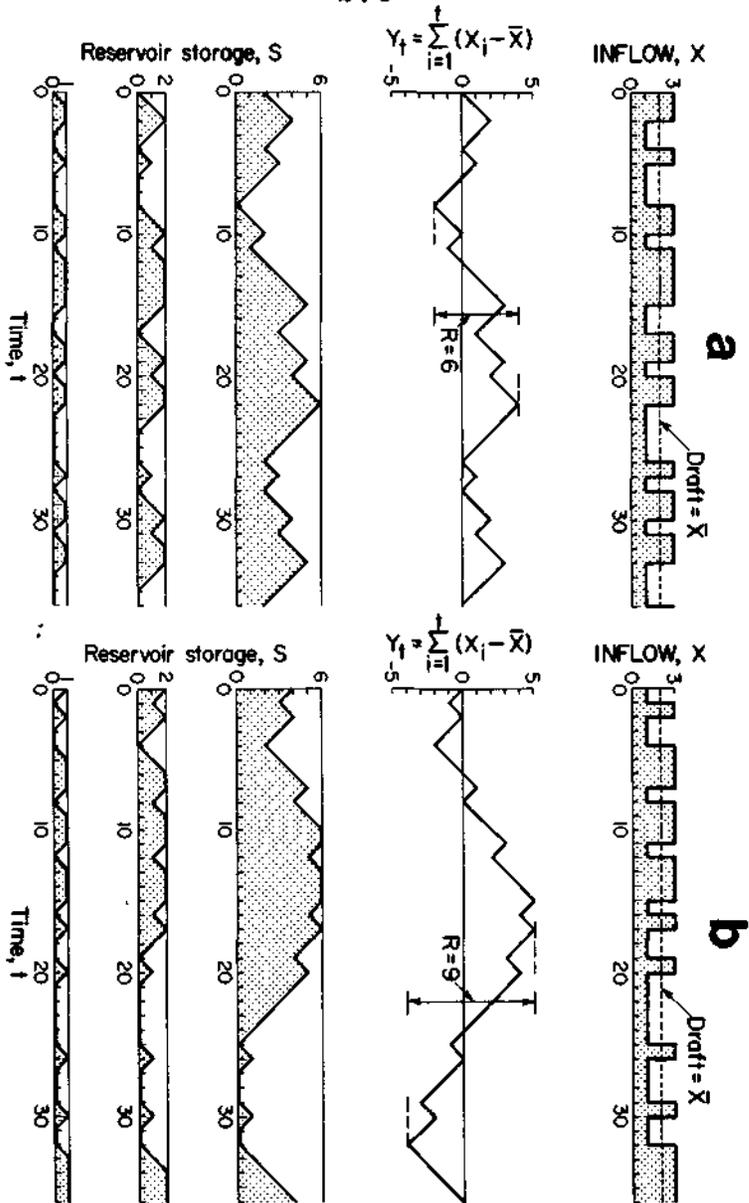
Fig. 2 Inflow series a and b (top); residual mass curves of series a and b (second from top); fluctuations of storage in reservoirs of storage capacity  $K = 6, 2$  and  $1$  subject to inflow series a and b and to draft  $Q = 2$  (lower half of the figure).
