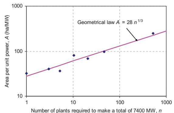
**Fig. 15** Graphical depiction of reservoir area per unit power vs number of plants required to make a total of 7400 MW. The data are from an inventory of 188 existing hydropower plants, classified into seven categories by installed power (from Goodland, 1995, quoted in Égré & Milewski, 2002). Each point represents the geometrical mean of each category, where 7400 MW is the geometrical mean of the first category (plants with largest installed power).
