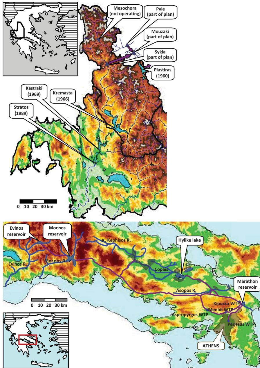
**Fig. 12** The two largest hydrosystems of Greece: (Upper) The Acheloos system with existing and planned projects annotated; violet arrows indicate the planned water transfer. (Lower) The Athens water supply system with the four reservoirs and the four water treatment plants (WTP) annotated; grey shaded areas indicate aquifers whose water is also transferred to Athens; violet lines represent the water transfer paths.
