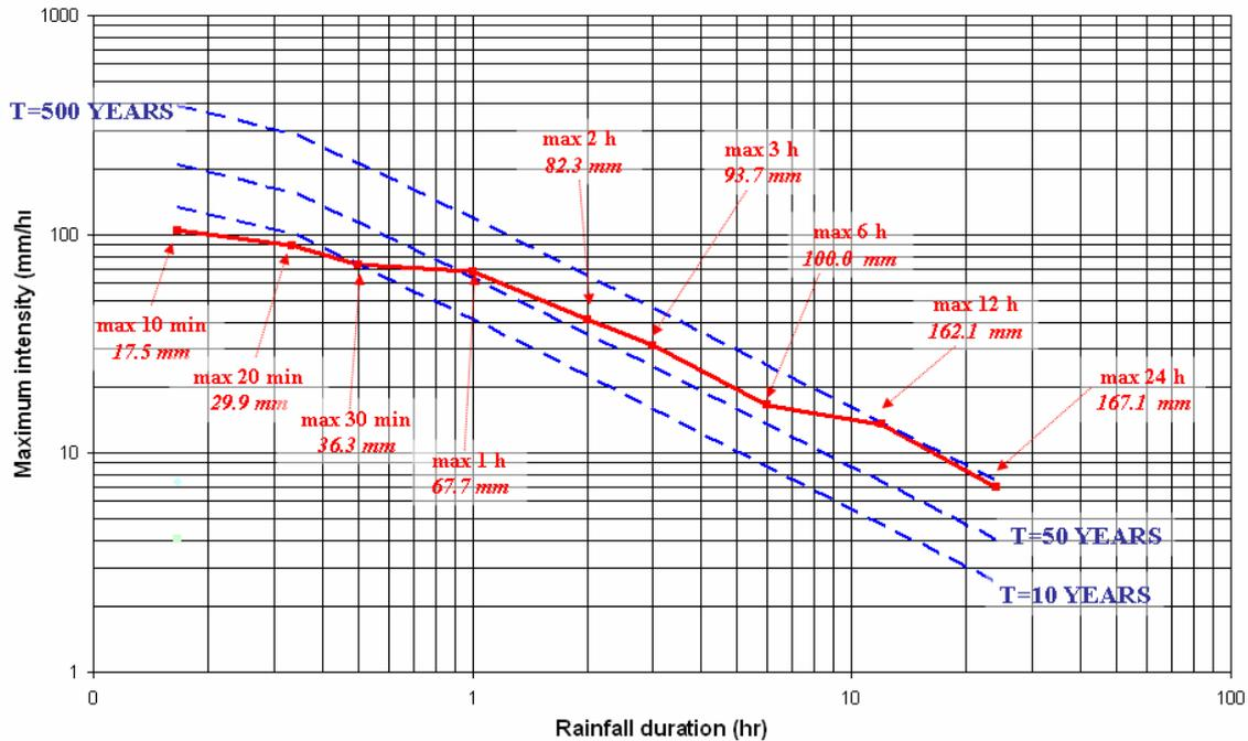
Fig. 10: Frequency analysis of the storm as measured in NTUA station
