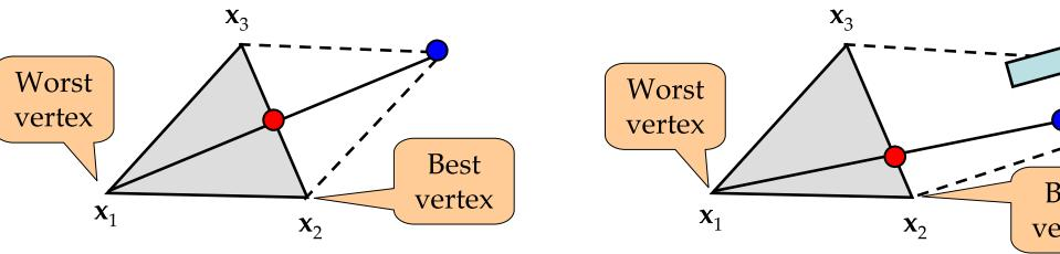
Reflection of the simplex through its centroid, according to the original Nelder-Mead (1965) procedure
