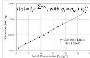
Figure 2: Light intensity attenuation factors (slope and intercept of the trend-line). Where C is the R6G concentration and x, the distance the laser beam travels through the water-tank (from pixel i to i-1).
