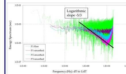
Figure 8: Energy spectra along the jet-axis.
