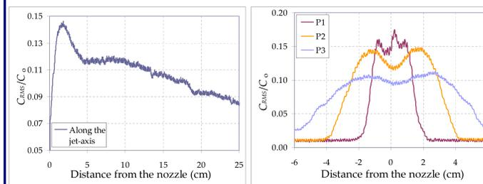
Figure 6a: Distribution of the RMS concentration along the jet-axis. Figure 6b: Distribution of the RMS concentration perpendicular to the jet-axis.
