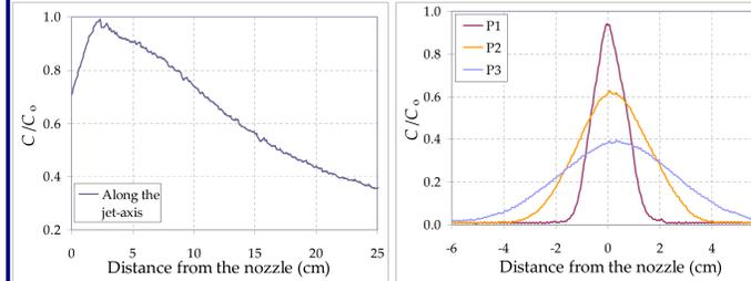
Figure 5a: Distribution of the concentration along the jet-axis. Figure 5b: Distribution of the concentration perpendicular to the jet-axis.
