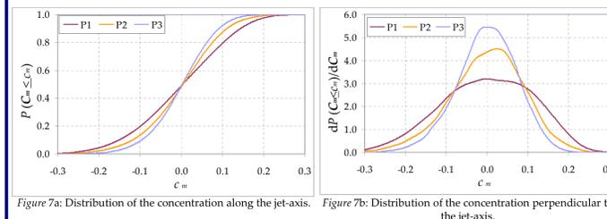
Figure 7a: Distribution of the concentration along the jet-axis. Figure 7b: Distribution of the concentration perpendicular to the jet-axis.
