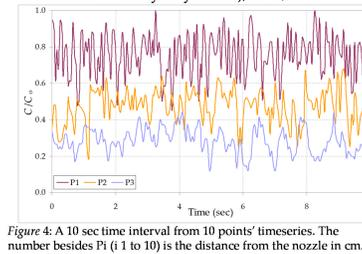
Figure 4: A 10 sec time interval from 10 points' timeseries. The number besides P1 (i 1 to 10) is the distance from the nozzle in cm.
