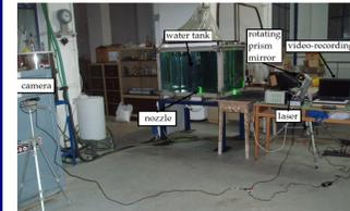
Figure 1: PLIF experimental set-up (NTUA, Laboratory of Hydraulics). The camera (for video tapping), nozzle, water-tank, rotating prism mirror, laser and video-recording (for video digitization) are shown.
