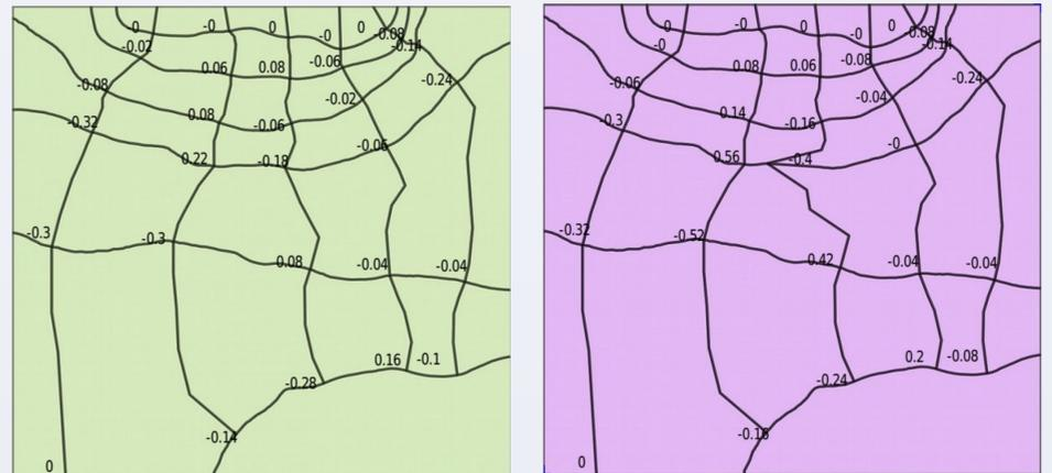
Original (left) and deformed (right) meshes with ratios of lateral to longitudinal fluxes.
