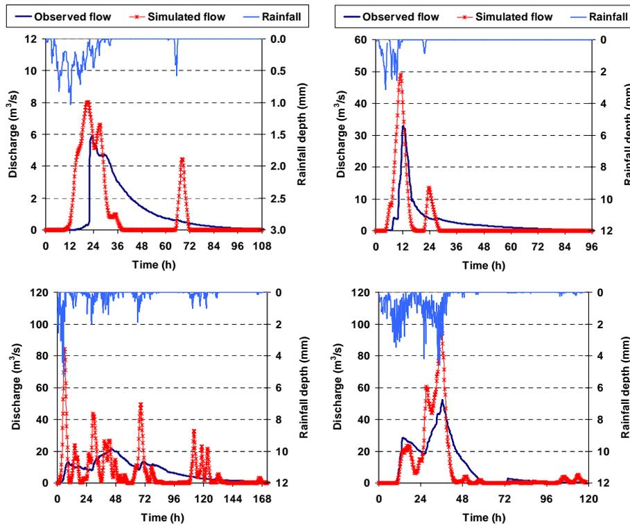
**Figure 1.** Observed and simulated (through the SCS/SUH method) hydrographs and corresponding rainfall events in Sarantapotamos (upper panel; February 2012, left, and February 2013, right) and Peristerona (lower panel; March 1988, left, and January 2004, right).
