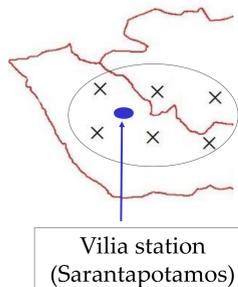
Estimation of station rainfall as weighted sum of the neighboring grid points, where the weights are estimated by minimizing the difference between the forecasted and observed rainfall volumes; next, estimation of areal rainfall over each sub-basin using the Thiessen polygon method to the forecasted values of the stations.
