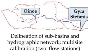
Delineation of sub-basins and hydrographic network; multisite calibration (two flow stations)
