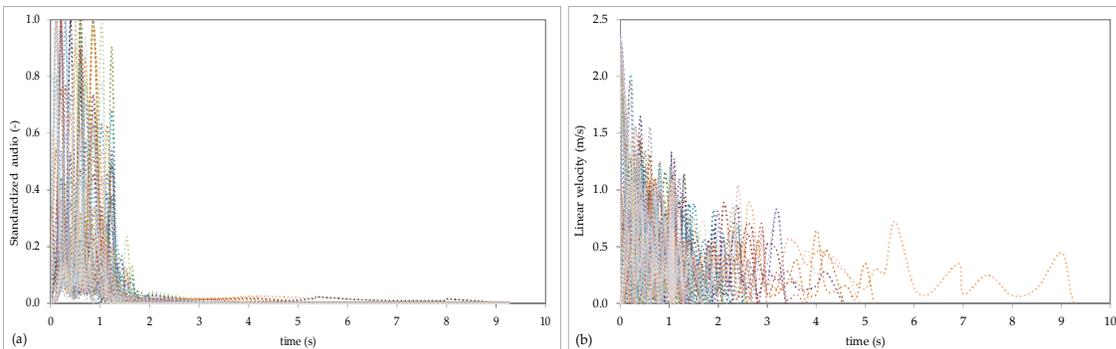
135 **Figure 3:** All experiments' (a) standardized audios, showing the time the die collides with the box (picks)
