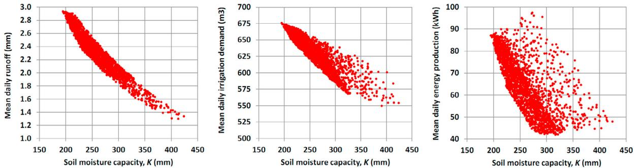
Fig. 8. (a) Mean daily runoff (output of hydrological model, input of reservoir model) vs. behavioural soil moisture capacity values; (b) Mean daily demand for irrigation (depends on simulated evapotranspiration deficits) vs. behavioural soil moisture capacity values; (c) Mean daily hydropower production vs. behavioural soil moisture capacity values
