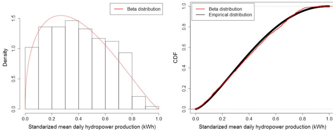
Fig. 7. Fitting of the Beta distribution to standardized mean daily hydropower production values.
