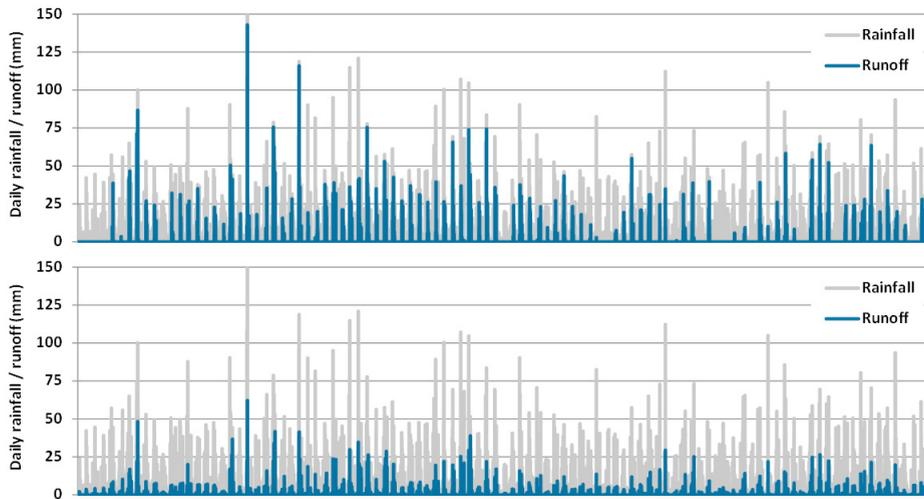
Fig. 6. Simulated runoff vs. synthetic rainfall assuming two extreme behavioural parameter sets (upper set:  $I_a = 57.8$  mm,  $K = 194.7$  mm,  $a = 0.00342$ ; lower set:  $I_a = 0.8$  mm,  $K = 424.2$  mm,  $a = 0.00157$ ).
