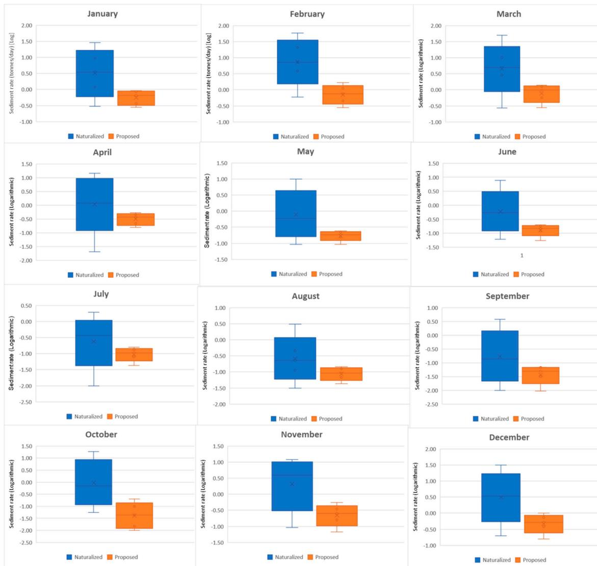
**Figure 8.** Monthly box plots for sediment rates at Mabine Station for natural conditions (observed data) and considering simulated data under the proposed EF policy (t/day, in logarithmic scale).
