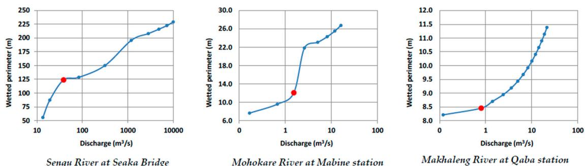
**Figure 4.** Semi-logarithmic plots of wetted perimeter vs. discharge at the three pilot sites of interest, highlighting the lowest breakpoint (change of slope).
