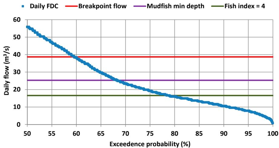
**Figure 6.** Comparison of flow-duration curve (blue line) of Senqu River at Seaka Bridge for 1995–2011 against critical flow thresholds defined in the context of EFA (the lower part of the curve is shown, corresponding to flows lower than the median, thus exhibiting exceedance probability >50%).
