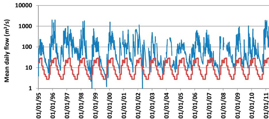
**Figure 5.** Daily flow time series of Senqu River at Seaka Bridge during 1995–2011 (semi-logarithmic plot) against monthly minimum baseflow values defined in the context of EFA.
