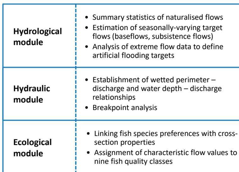
**Figure 2.** Flowchart of the proposed EFA framework.
