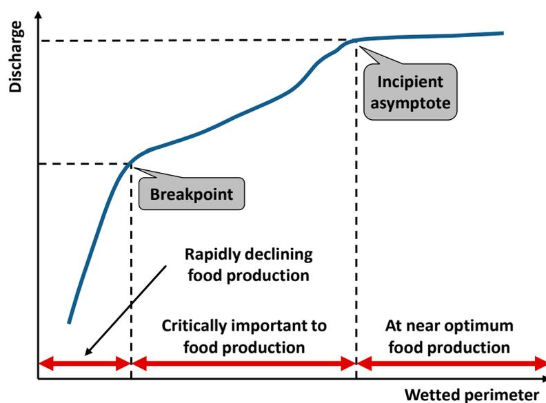
**Figure 3.** Example of wetted perimeter–discharge curve showing relationship between breakpoints and fish food production (adapted by CDFW [21]).
