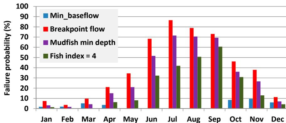
**Figure 7.** Monthly failure probabilities (%) using four flow categories defined in the context of EFA.
