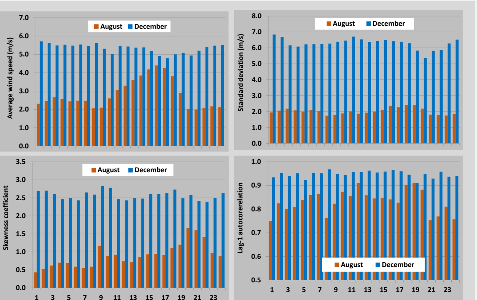
Plots of intra-daily (i.e., hourly) statistical characteristics of wind speed data at Ikaria for two characteristic months (August, December)
