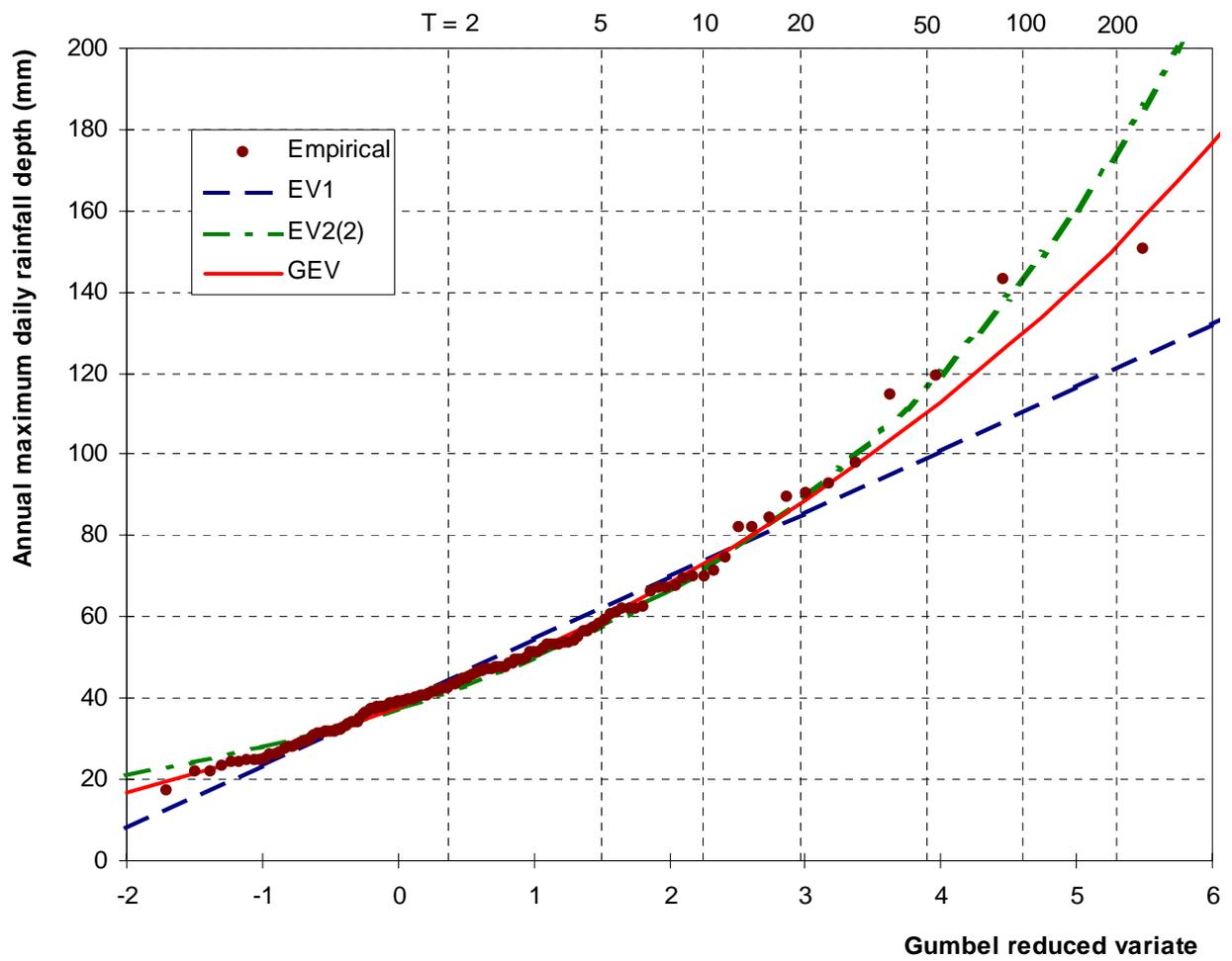
**Figure 4** EV1, EV2(2), and GEV distributions fitted to the sample of annual maximum daily rainfall depths by the method of L-moments, in comparison with the empirical distribution estimated using Gringorten plotting positions.
