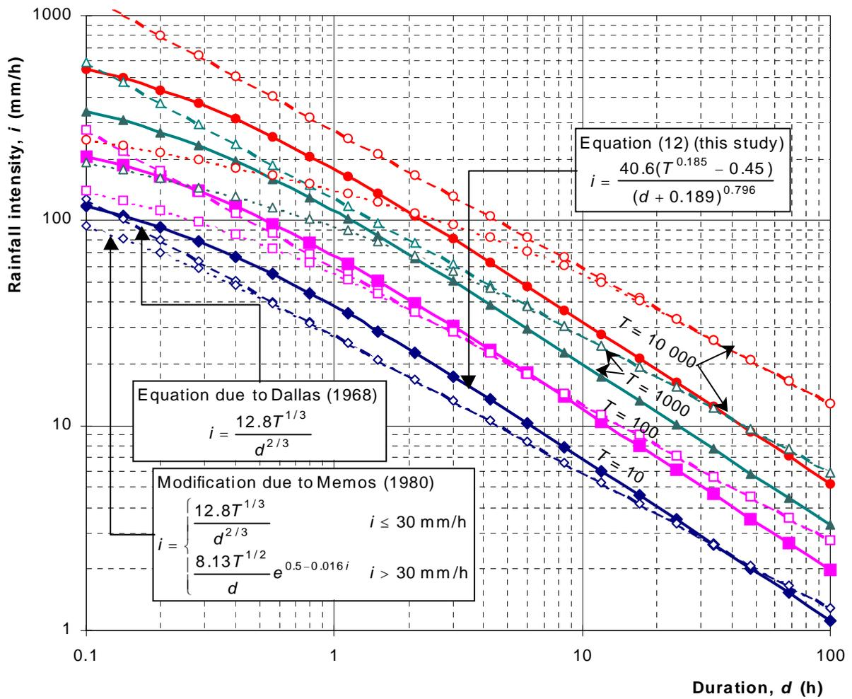
**Figure 7** Comparison of intensity-frequency duration curves for Athens derived in this study (solid curves; eqn. (12)) with earlier empirical idf curves of the same region.
